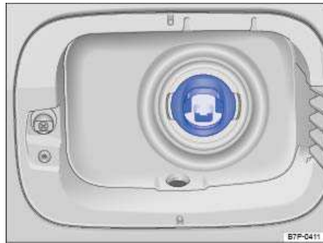
Fig. 136 With open fuel cap: Misfueling guard in the fuel filler neck.
