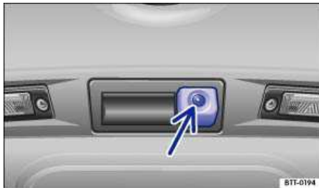
Fig. 127 In the luggage compartment lid: Location of the Rear Assist camera.
