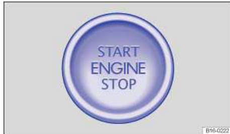
Fig. 112 In the center console: Starter button for the Keyless Access locking and starting system.
