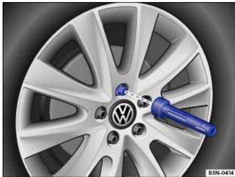
Fig. 167 Changing a wheel: Remove previously loosened wheel bolts using the screwdriver handle.
