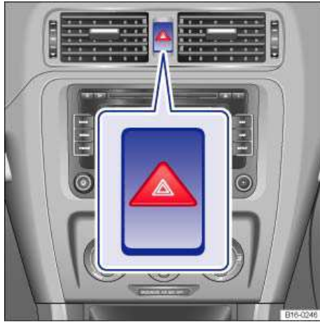
Fig. 148 In the center of the instrument panel: Button for the emergency flashers.
