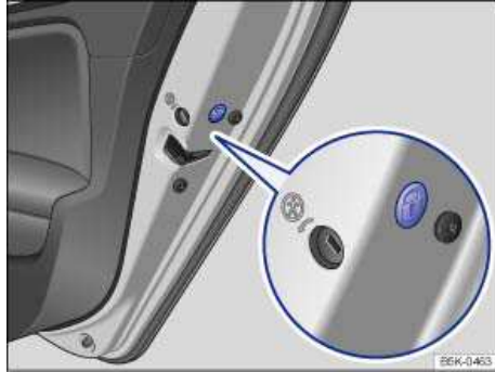
Fig. 150 On the front side of the right rear door: Emergency lock, covered by a rubber seal.
