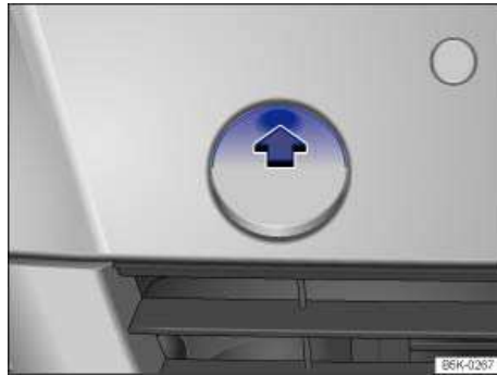
Fig. 181 In the right front bumper: Removing the cover.
