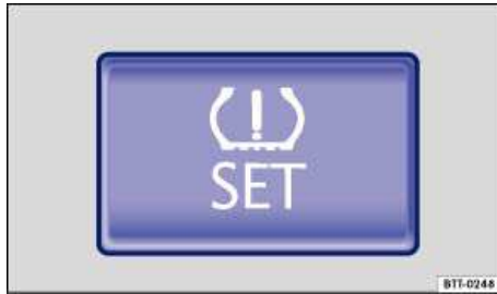
Fig. 94 In the glove compartment: SET button for the Tire Pressure Monitoring System.
