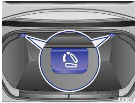
Fig. 81 On the left side of the luggage compartment: Release lever for the left-side rear seat backrest. The release lever for the right-side rear seat backrest is on the right side of the luggage compartment.
