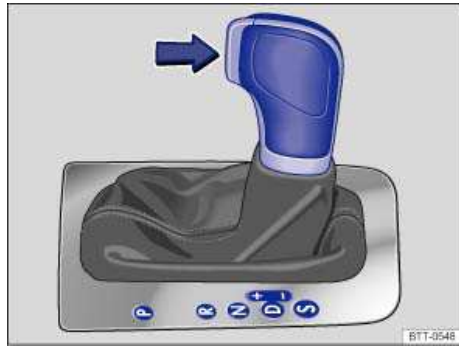
Fig. 119 Side view: Automatic transmission selector lever with shift lever release button (arrow).
