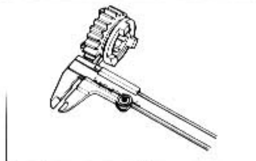
Checking groove width
