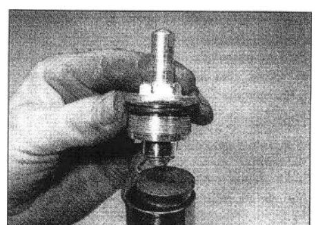
7.27 Fit a new O-ring onto the top bolt and thread the bolt into the fork tube
