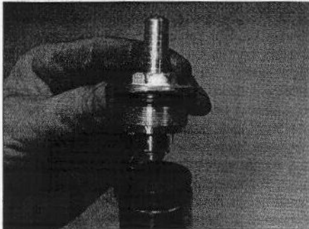
29.2 Unscrew the fork top bolt
