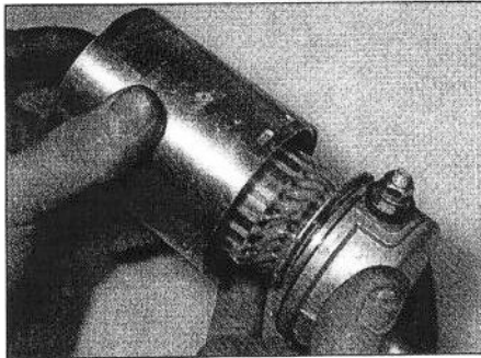
30.19 . . . and the main housing over the armature
