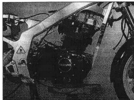
5.17 Support the engine using a jack and a block of wood
