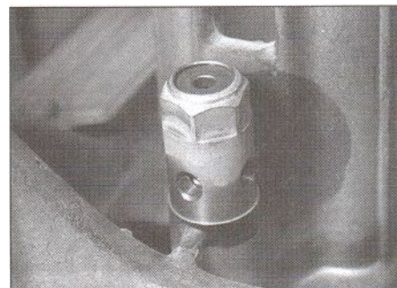
22.12 Oil pressure regulator location
