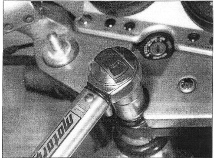
8.14 Tighten the steering stem bolt to the specified torque setting
