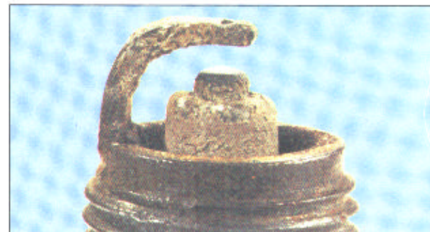
Worn plug – Worn electrodes will cause poor starting in damp or cold weather and will also waste fuel
