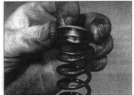
29.6a Fit the spring seat, shouldered side down, into the top of the spring, then install the spring into the fork tube . . .
