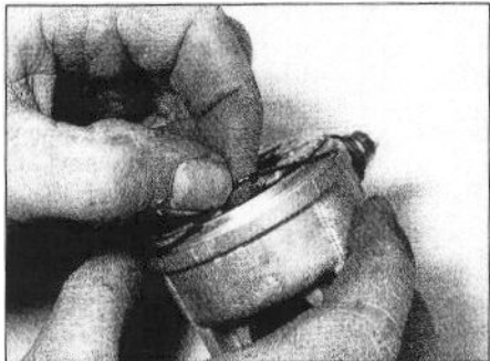
30.17 Fit a new O-ring around the cover
