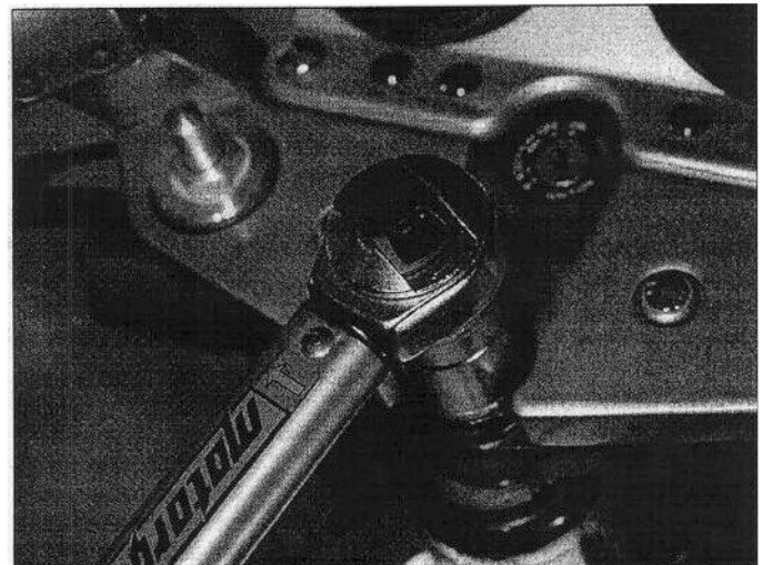
16.8 Tighten the steering stem bolt to the specified torque setting
