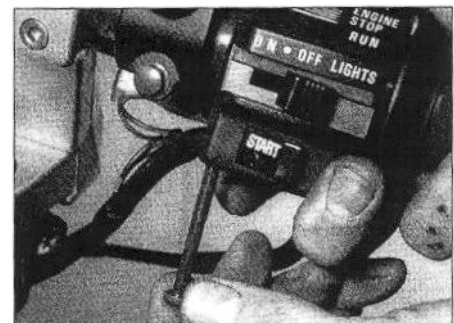
21.2 The switch is secured by two screws
