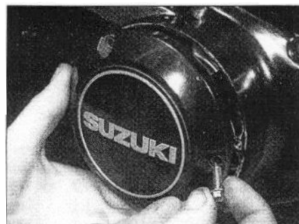
4.16 Install the pulse generator assembly cover
