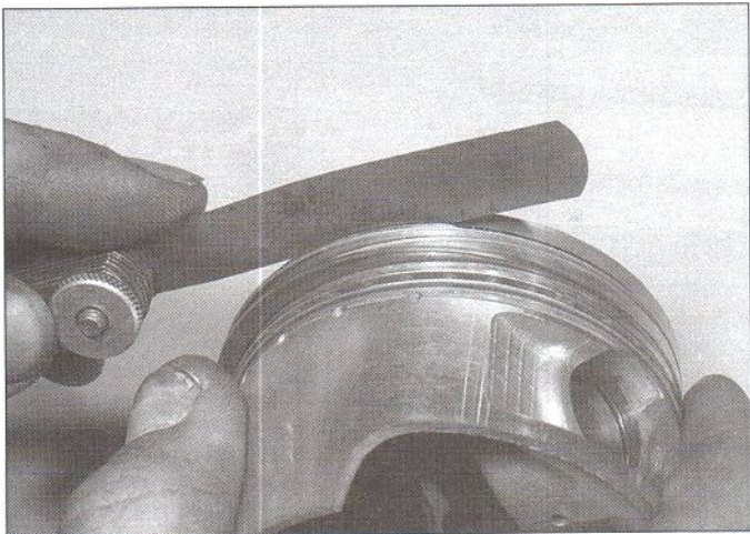
15.11 Measure the piston ring-to-groove clearance with a feeler gauge
