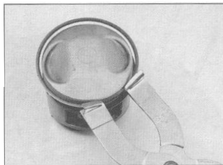
15.5a Removing the piston rings using a ring removal and installation tool
