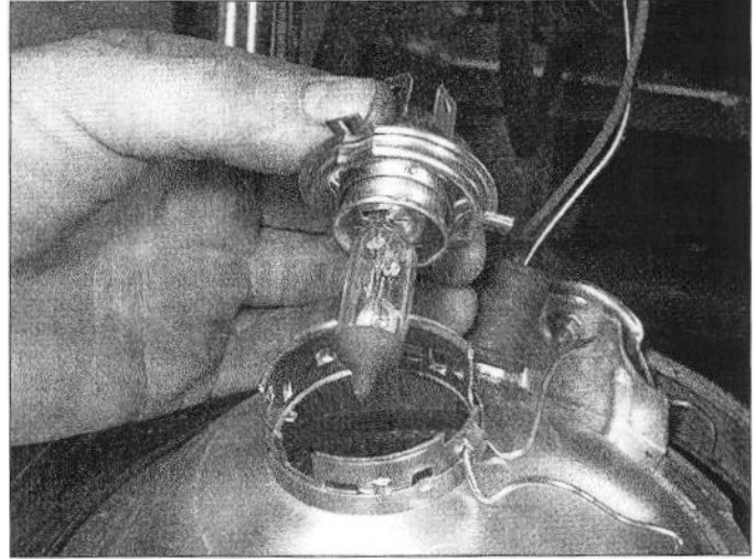
7.3b . . . and remove the bulb
