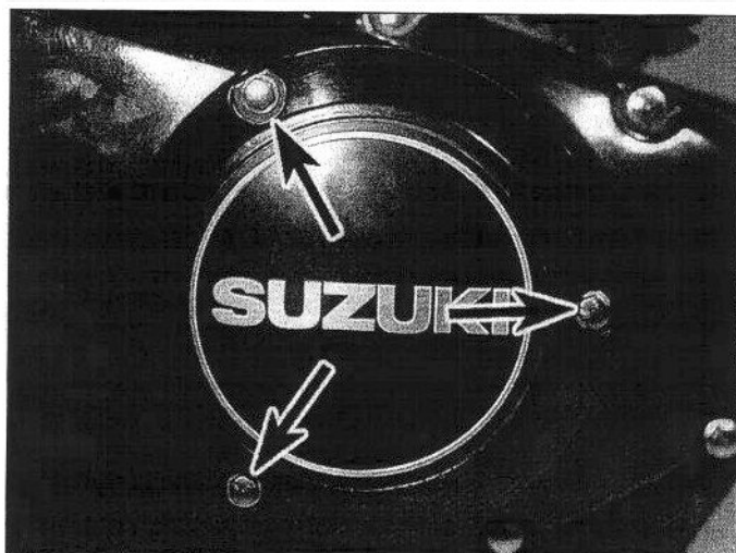
10.2a The pulse generator cover is secured by three screws (arrows)
