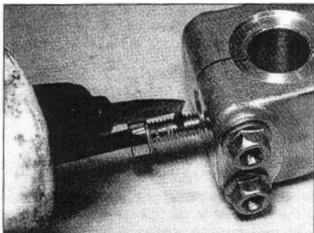
7.20b Apply thread locking compound to the damper rod bolt and use a new sealing washer
