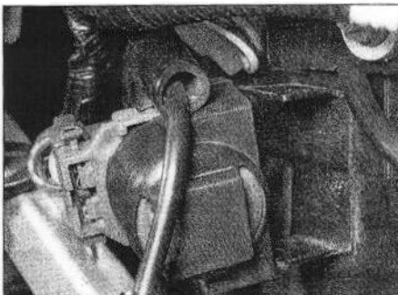
28.8 The relay's rubber sleeve mounts onto lugs on the frame
