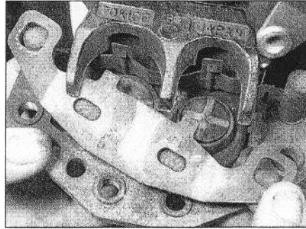
2.9b Fit the inner pad onto its guide pins . . .
