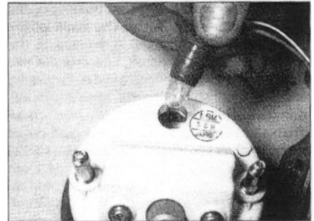
16.4b ... and remove the bulbholder
