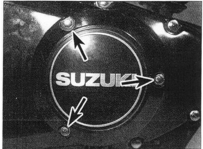
4.7 The pulse generator coil assembly cover is secured by three bolts
