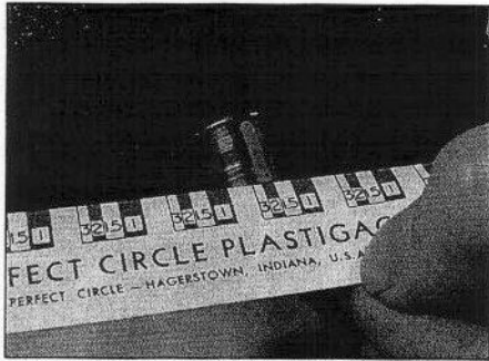
10.16 Measure the crushed Plastigauge using the scale on the pack to obtain the oil clearance
