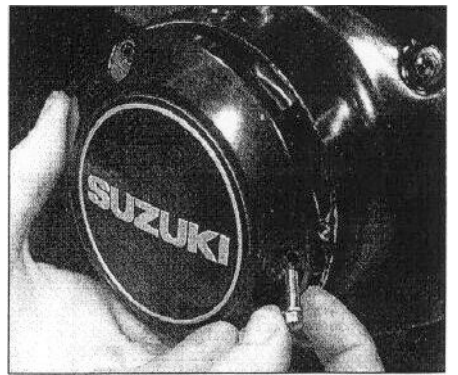
17.27 Install the pulse generator assembly cover
