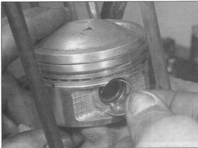
15.17 Always use new circlips to secure the piston pin
