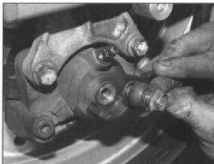
5.20 Use a new sealing washer on each side of the union
