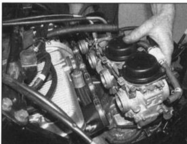
7.7b . . . and ease the carburettors back out of the intake ducts
