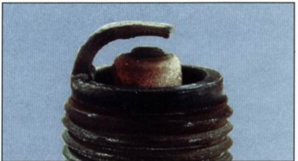
Worn plug – Worn electrodes will cause poor starting in damp or cold conditions and will also waste fuel.
