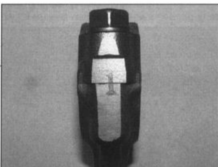
28.3 This number indicates the connecting rod bearing size and faces to the back – make your own marks to indicate cylinder number
