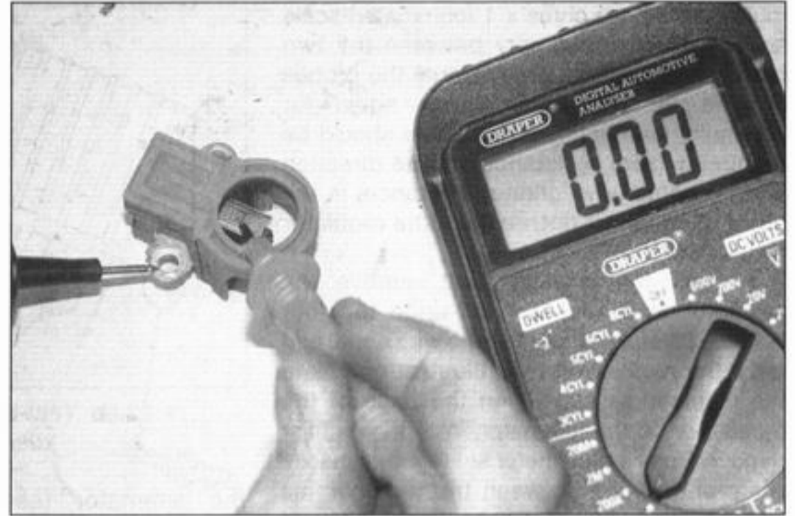
33.3c Check for continuity between each brush and the mounting plate
