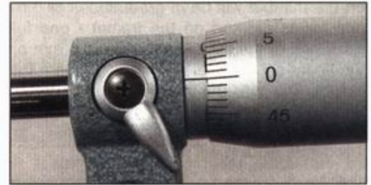
3.2 Check micrometer calibration before use
