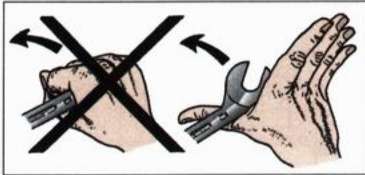
4.6 If you can't pull on the spanner to loosen a fastener, push with your hand open
