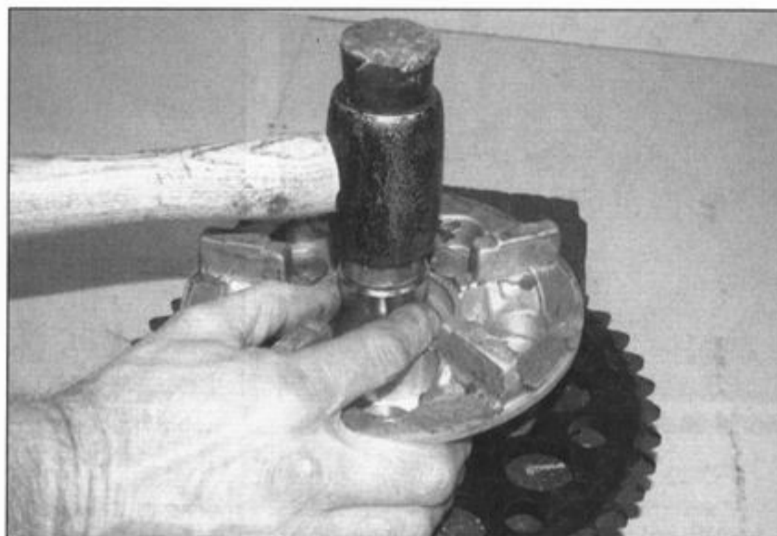
14.23 Drive the bearing out as described
