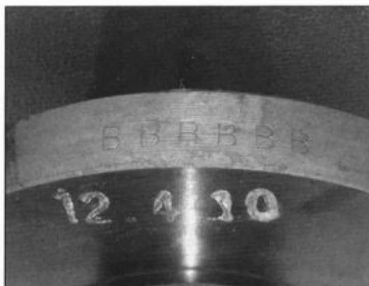
27.23a Crankshaft main bearing journal size letters
