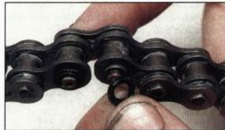
8.5 . . . install the O-rings over the pin ends . . .
