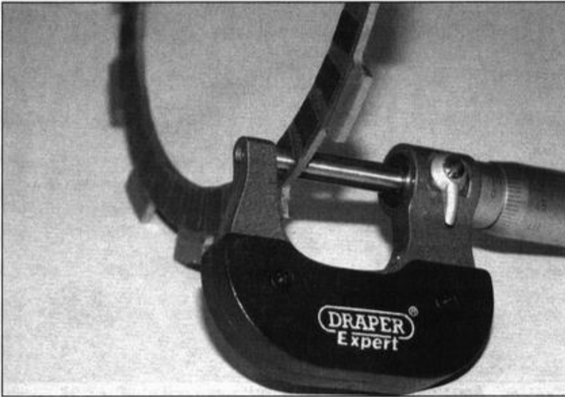
18.12 Measure the thickness of the friction plates . . .
