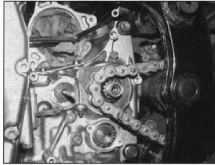
5.23b Slip the chain off the end of the shaft when possible . . .
