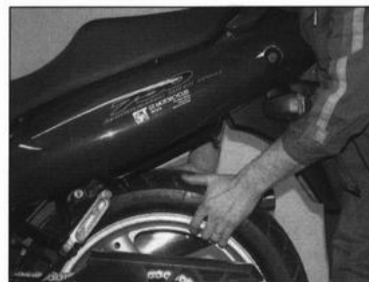
20.8 Checking for play in the rear shock mountings and suspension linkage bearings
