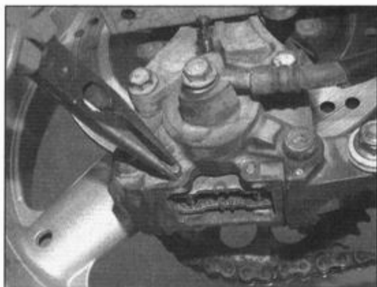
2.16 Withdraw the pad pins and remove the springs and pads
