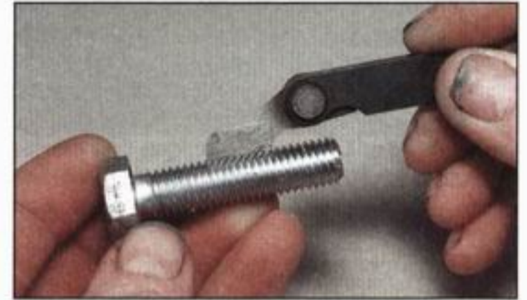
2.12 Using a thread gauge to measure pitch
