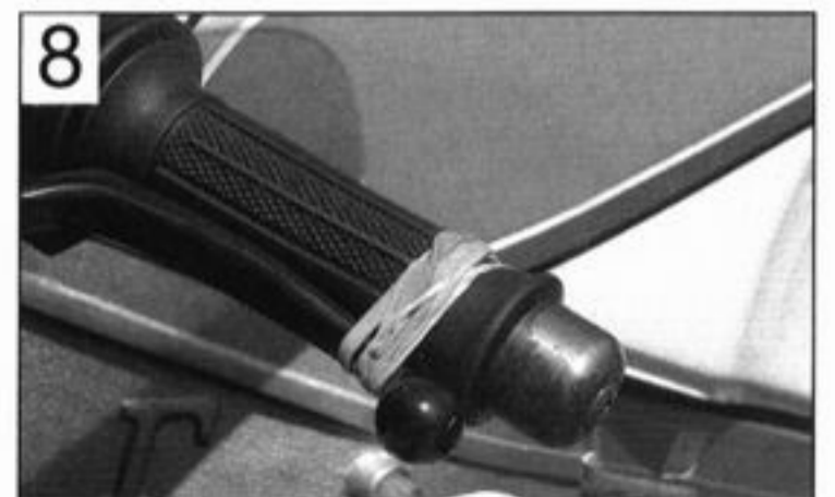
Hold clutch lever back against the handlebar with elastic bands or a cable tie
