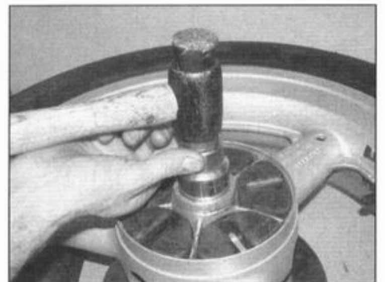
14.16 A socket can be used to drive in the bearing
