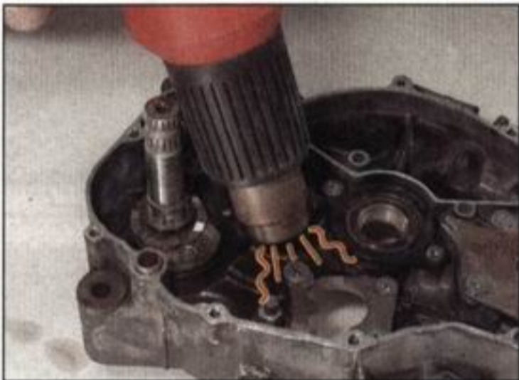
2.15 Using heat to free a seized fastener
