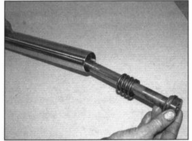
8.18a Slide the damper rod into the tube and all the way down so that it projects from the bottom . . .
