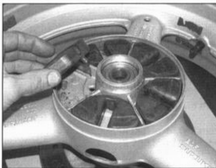
19.3 Check the rubber dampers
