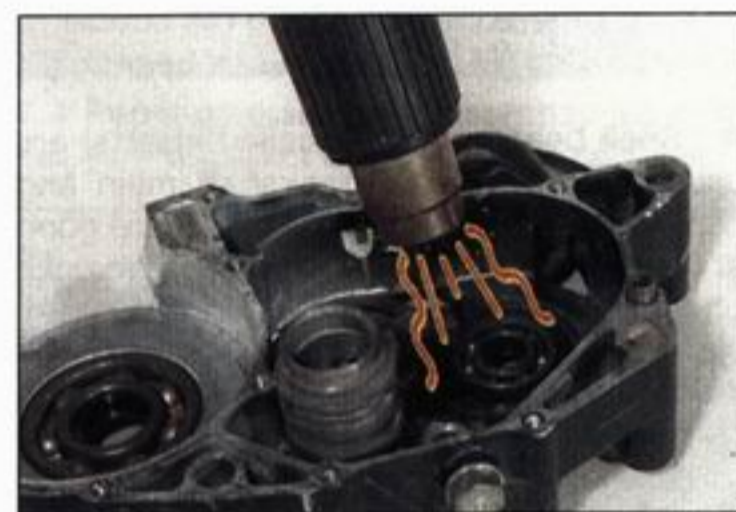
5.13 Using a localised heat source to aid bearing removal
