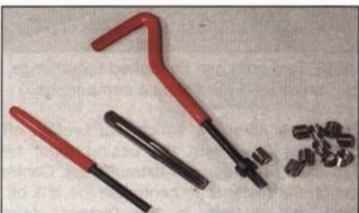
2.25 Obtain a thread insert kit to suit the thread diameter and pitch required
