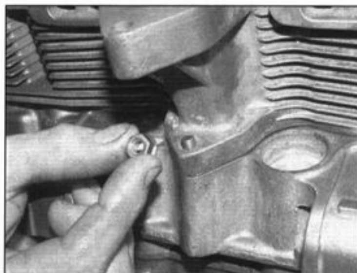
15.26 Install the single nut and tighten it to the specified torque setting
