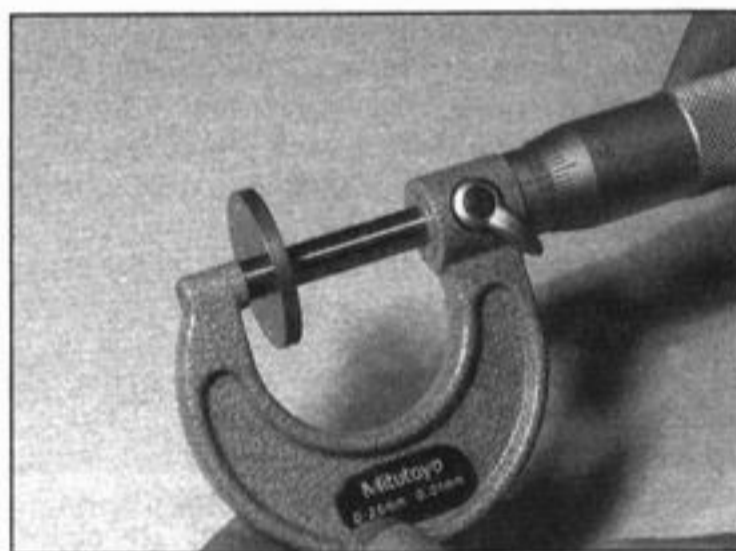
Tappet shims are measured with a micrometer
