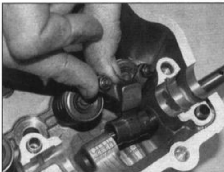
11.44b . . . followed by the rocker arm, then slide the shaft part-way through . . .
