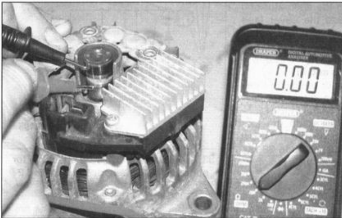
33.4a Check for continuity between the slip rings
