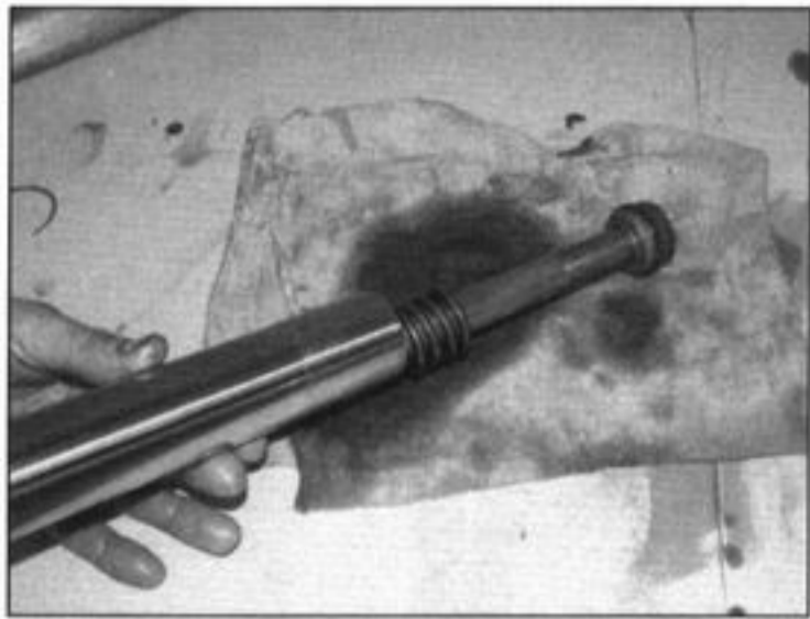
8.7b . . . then tip the damper rod out of the fork
