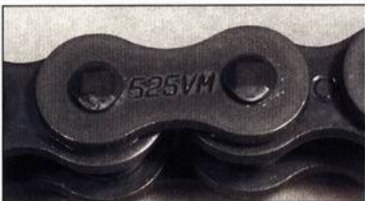
8.10 Typical chain size and type marking
