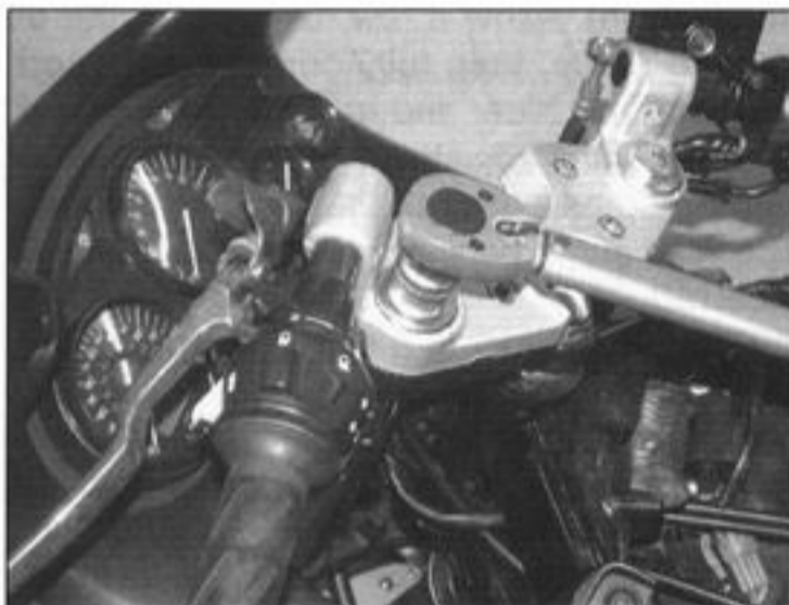
6.9a If required tighten the fork top bolt to the specified torque
