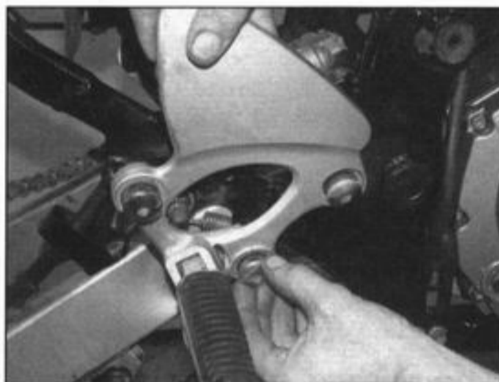
12.6a Unscrew the bolts and remove the footrest bracket (GSX750F model shown) . . .
