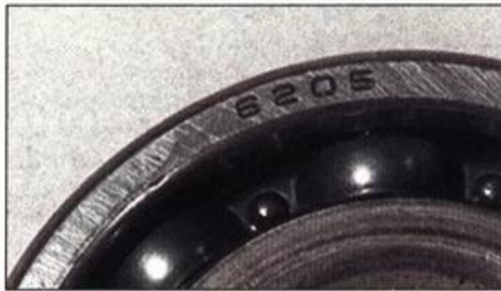
5.16 Typical bearing marking
