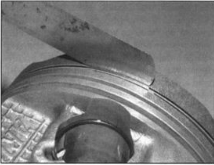
16.10 Measuring the piston ring-to-groove clearance with a feeler gauge
