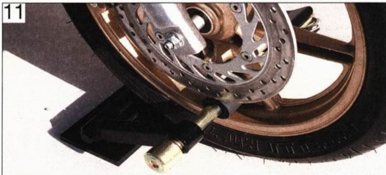
11 Permanent ground anchors provide an excellent level of security when the bike is at home
