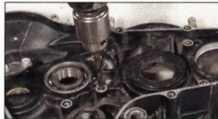
2.26 To install a thread insert, first drill out the original thread . . .
