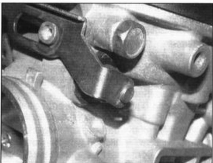
10.15b . . . locating the arms behind the plunger ends . . .
