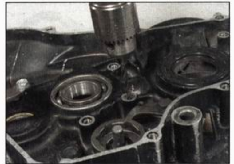
2.19 When using a screw extractor, first drill a hole in the fastener . . .
