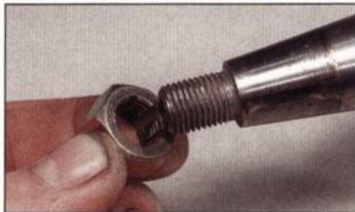
2.23 A thread repair tool being used to correct an external thread
