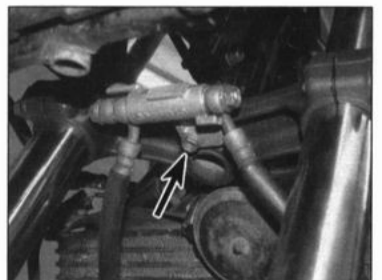
9.4 Unscrew the bolt (arrowed) and displace the brake hose splitter
