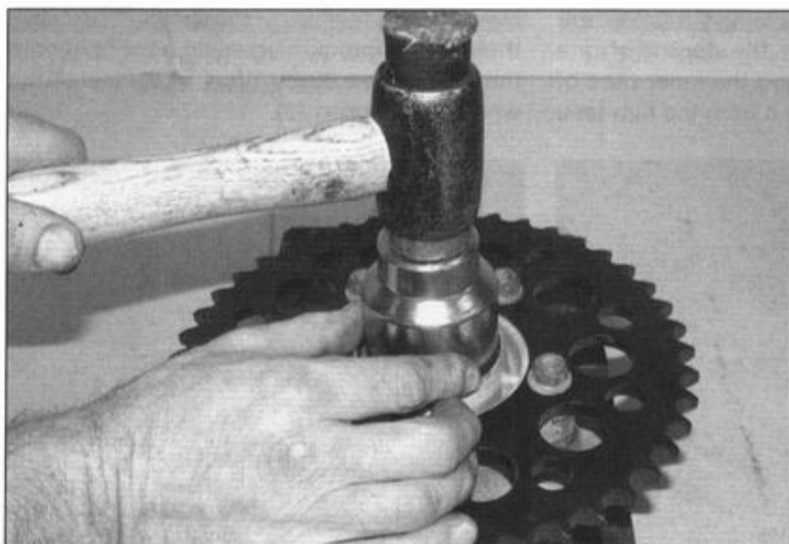
14.24 A socket can be used to drive in the bearing
