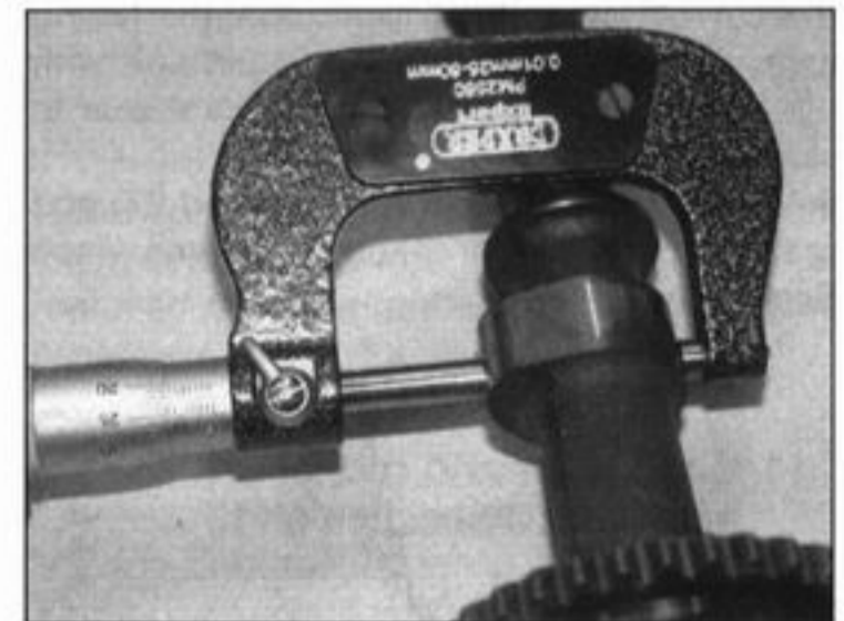
11.12 Measure the height of each lobe with a micrometer
