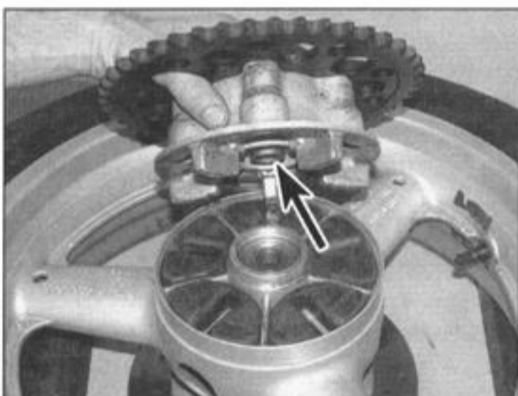
14.9 Lift the sprocket coupling out of the wheel, noting the spacer (arrowed)
