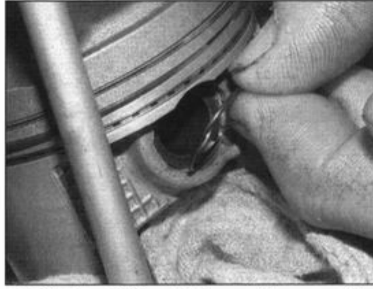
16.17b Install the circlip, making sure it is properly seated in its groove, with the open end away from the notch
