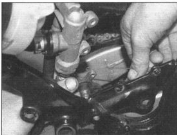
7.8d ... and unhook the brake light switch spring
