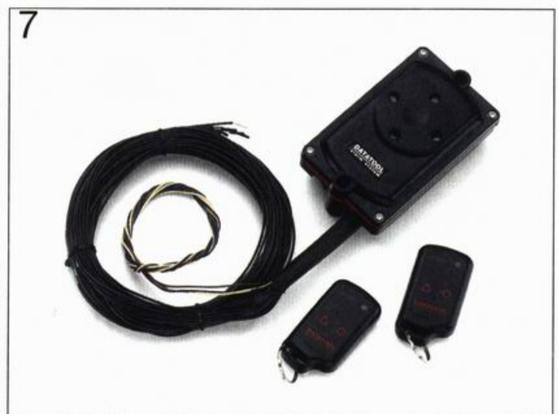
A typical alarm/immobiliser system
