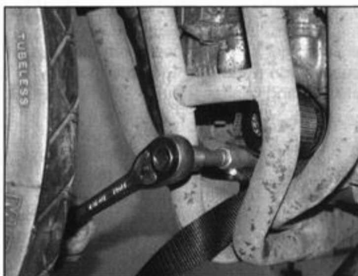
22.2a Unscrew the filter using a filter removing tool . . .
