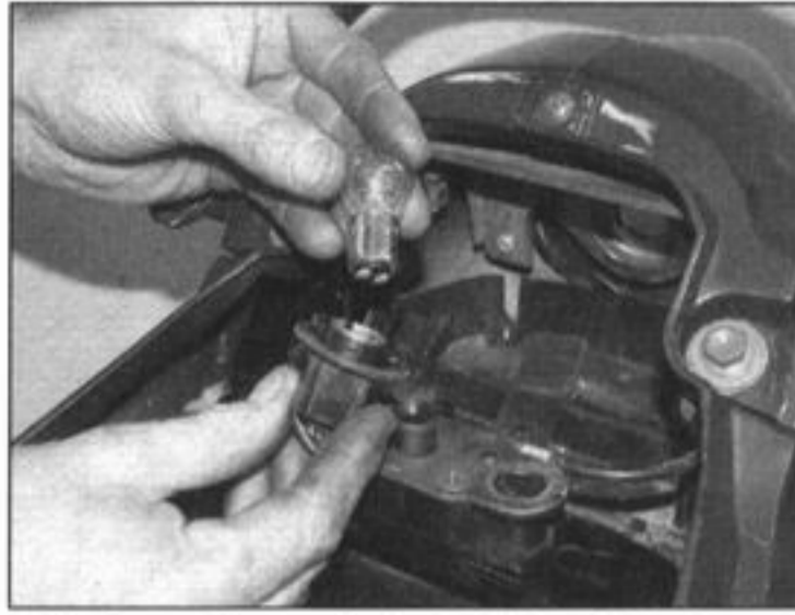
9.3 Carefully push the bulb in slightly and twist it anti-clockwise to release it
