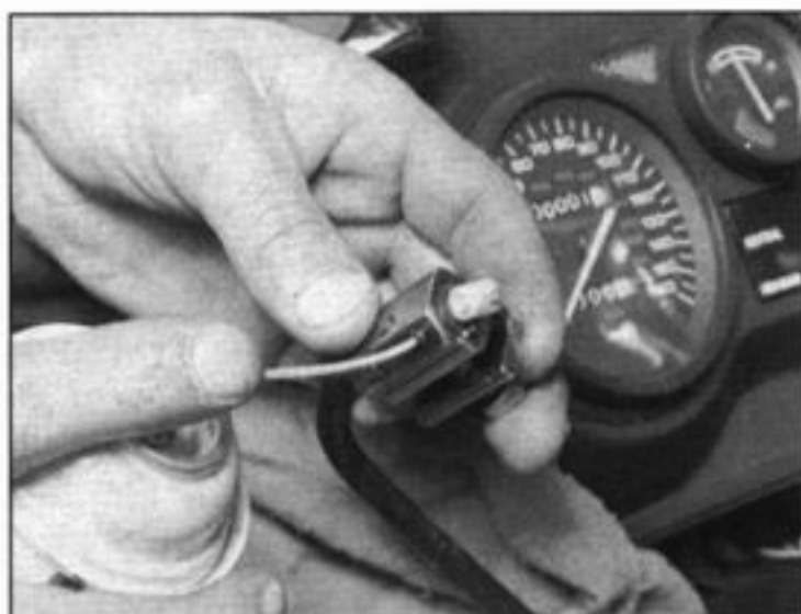
14.3a Lubricating a cable with a pressure lubricator. Make sure the tool seals around the inner cable
