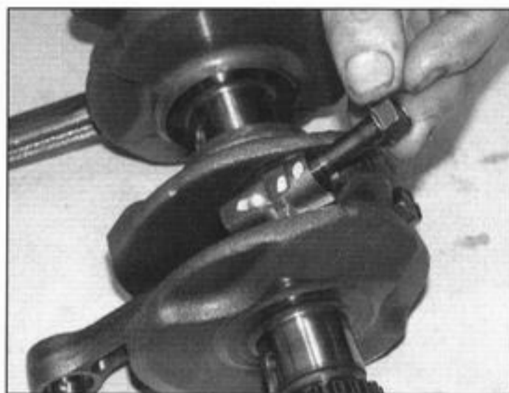
28.23 Install the bolts – 750 cc engine, or nuts – 600 cc engine . . .
