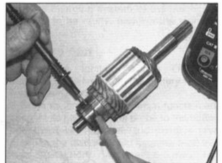
30.8a Continuity should exist between the commutator bars
