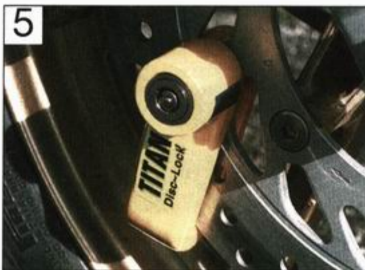
A typical disc lock attached through one of the holes in the disc
