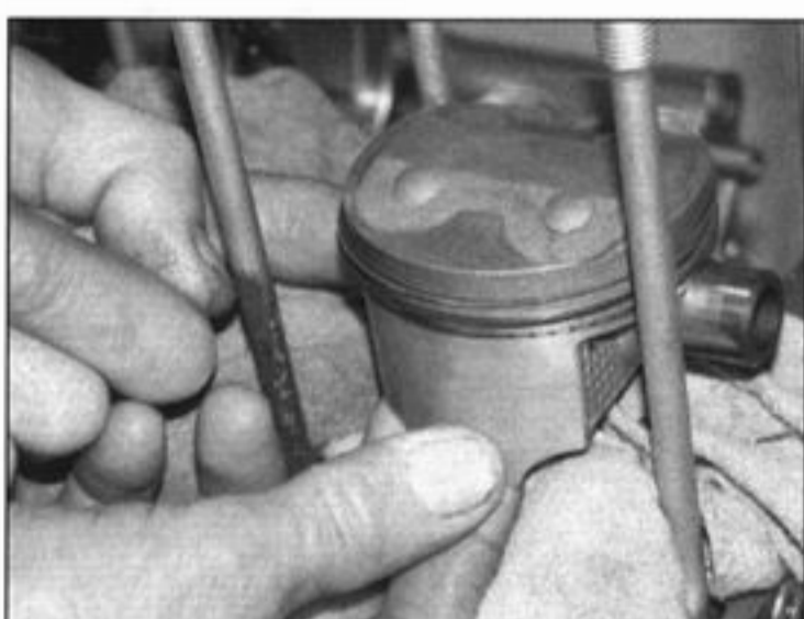
16.3b . . . then push the pin out from the other side and remove the piston
