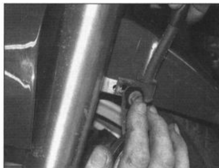
6.2 Unscrew the bolt and detach the brake hose from the fork
