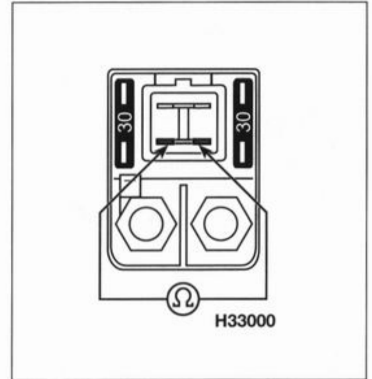
28.6 Measuring the relay coil resistance
