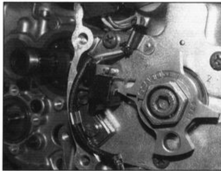
16.5b . . . until the scribe line aligns with the sensor on the coil . . .
