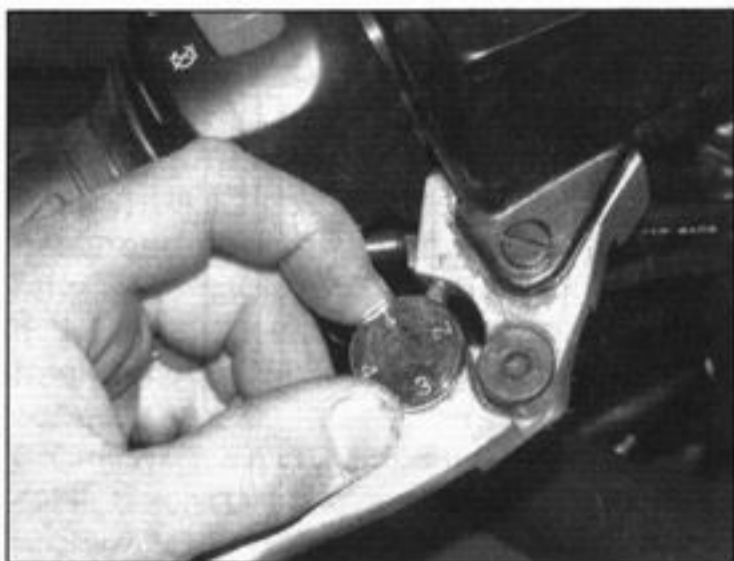
11.6 Adjusting the front brake lever span
