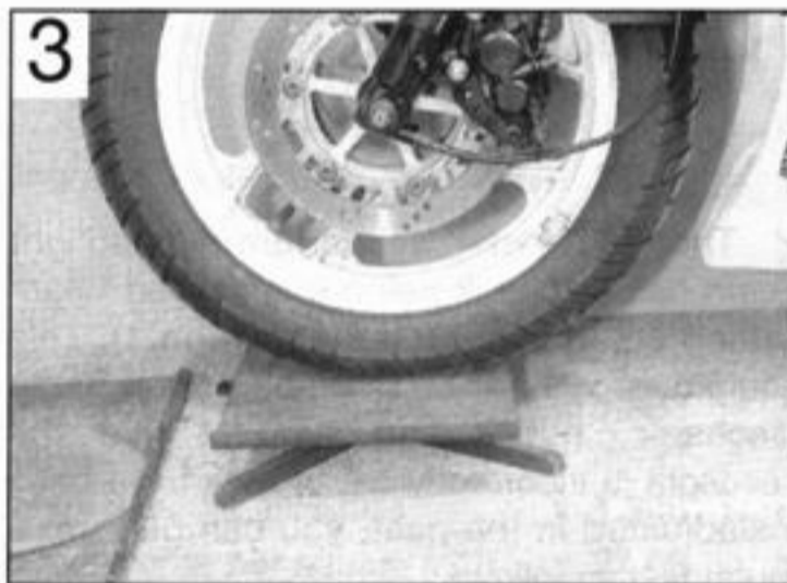
Front wheel mounted on a surface plate for steering head bearing lower race check
