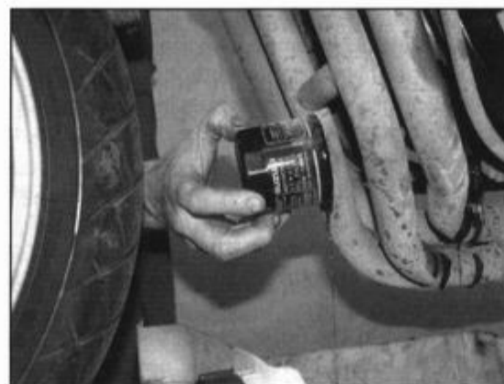
22.2b . . . and allow the oil to drain
