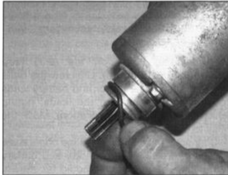
29.5 Fit a new O-ring smeared with grease
