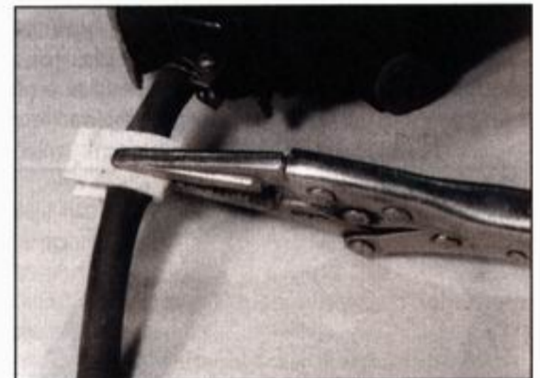
9.4 ... or thick card and self-locking grips
