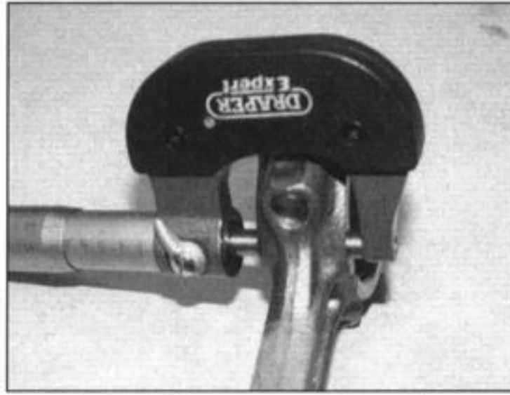
28.8a Measure the width of the connecting rod . . .
