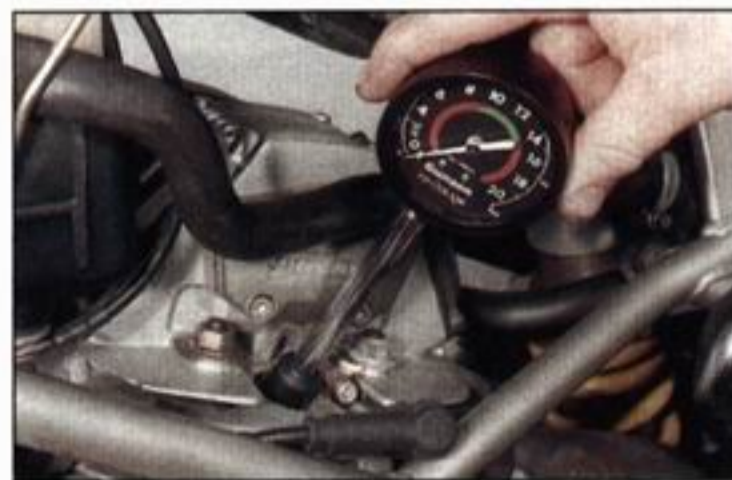
3.20 Using a rubber-cone type cylinder compression gauge
