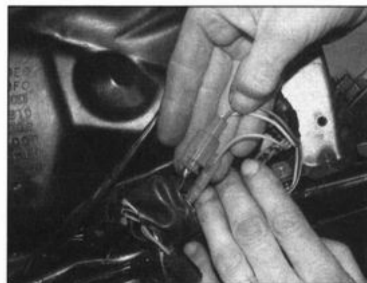
4.8 Disconnect the pulse generator coil wiring connector and the oil pressure switch bullet connector
