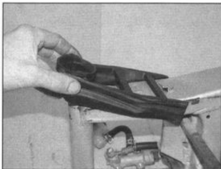
15.3 Chain slider locates in clip and over pivot boss
