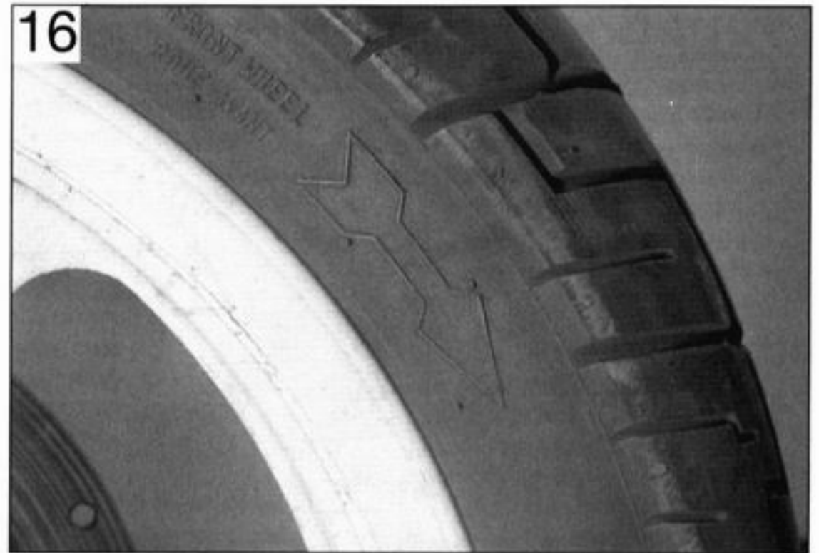
Tyre direction of rotation arrow can be found on tyre sidewall
