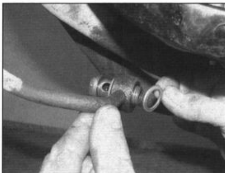
7.5 Always use new sealing washers on the banjo connections
