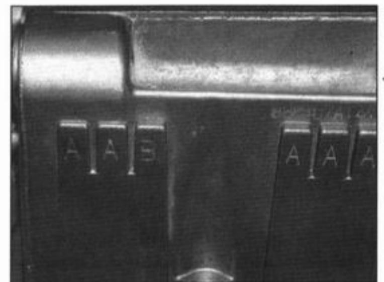
27.23b Crankshaft main bearing housing size letters
