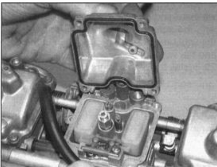
10.9 Fit a new sealing-ring into the groove and install the float chamber
