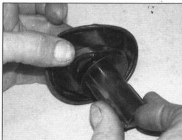
8.34 Peel the diaphragm off the piston and replace it with a new one
