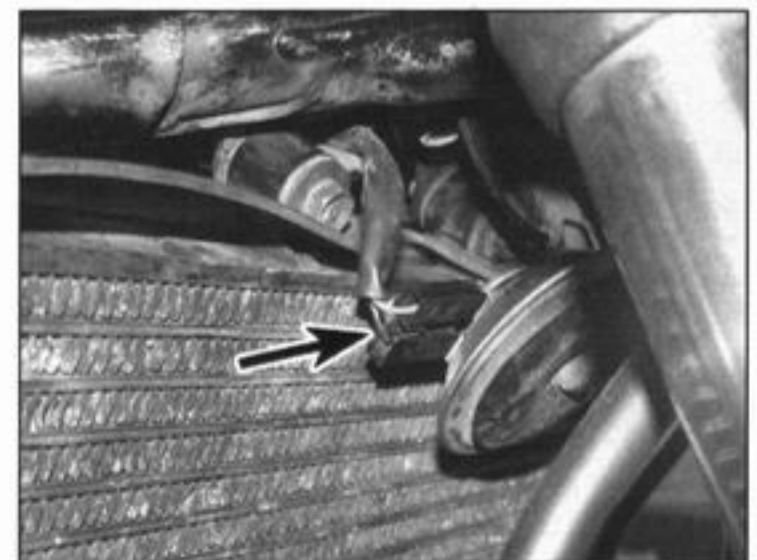
27.2 Horn wiring connectors (arrowed)
