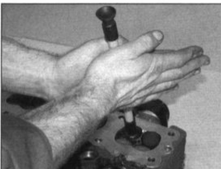
14.24 Rotate the valve grinding tool back and forth between the palms of your hands
