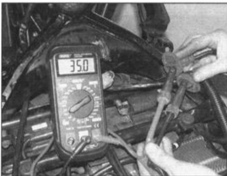
3.5 To test the coil secondary resistance, connect the multimeter leads to the spark plug sockets
