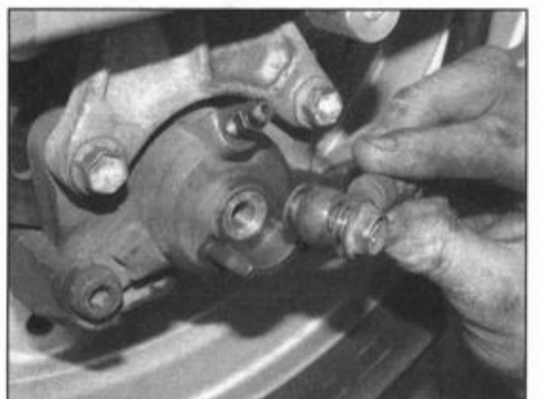
14.20 Use a new sealing washer on each side of the union
