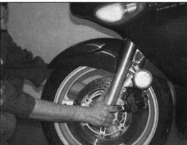
19.4 Checking for play in the steering head bearings
