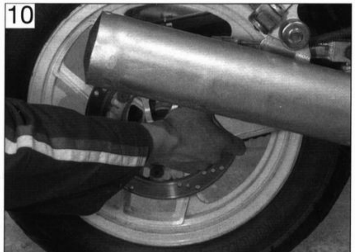
Grasp the swingarm at the ends to check for play in its pivot bearings
