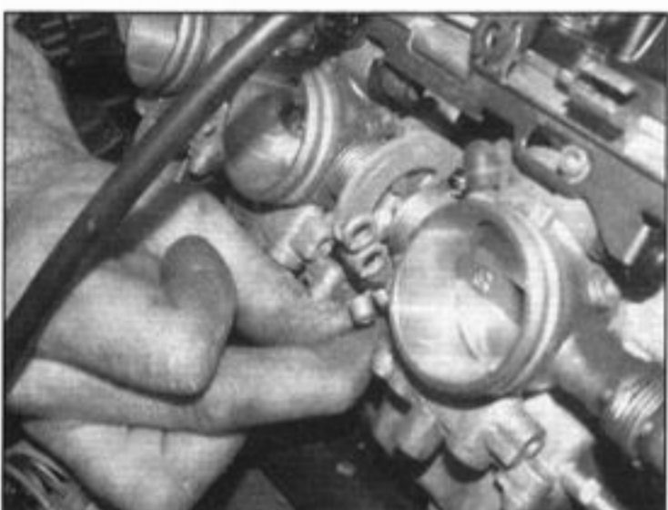
12.10b ... then fit the end into the cam
