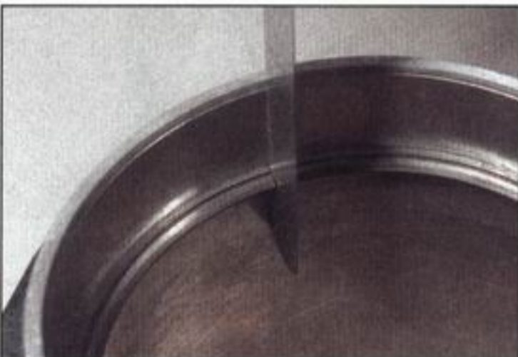
3.1 Feeler gauges are used for measuring small gaps and clearances - thickness is marked on one face of gauge
