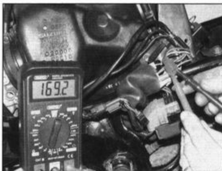
4.4 Check the resistance of the pulse generator coil
