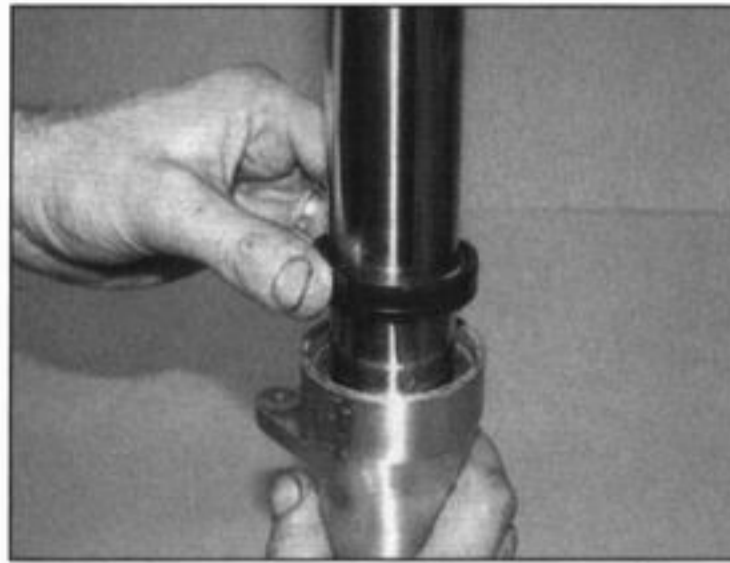
8.22 Smear the new oil seal with clean fork oil then slide it down the tube
