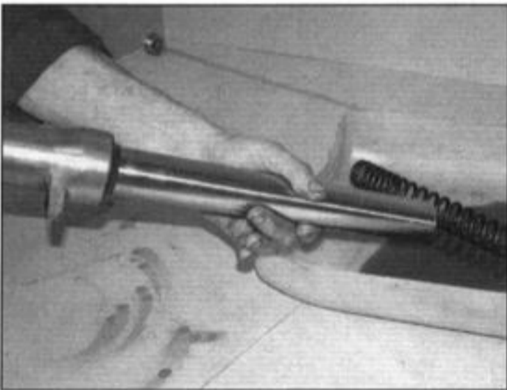
7.5 Invert the fork over a container and pump the tube to expel the oil
