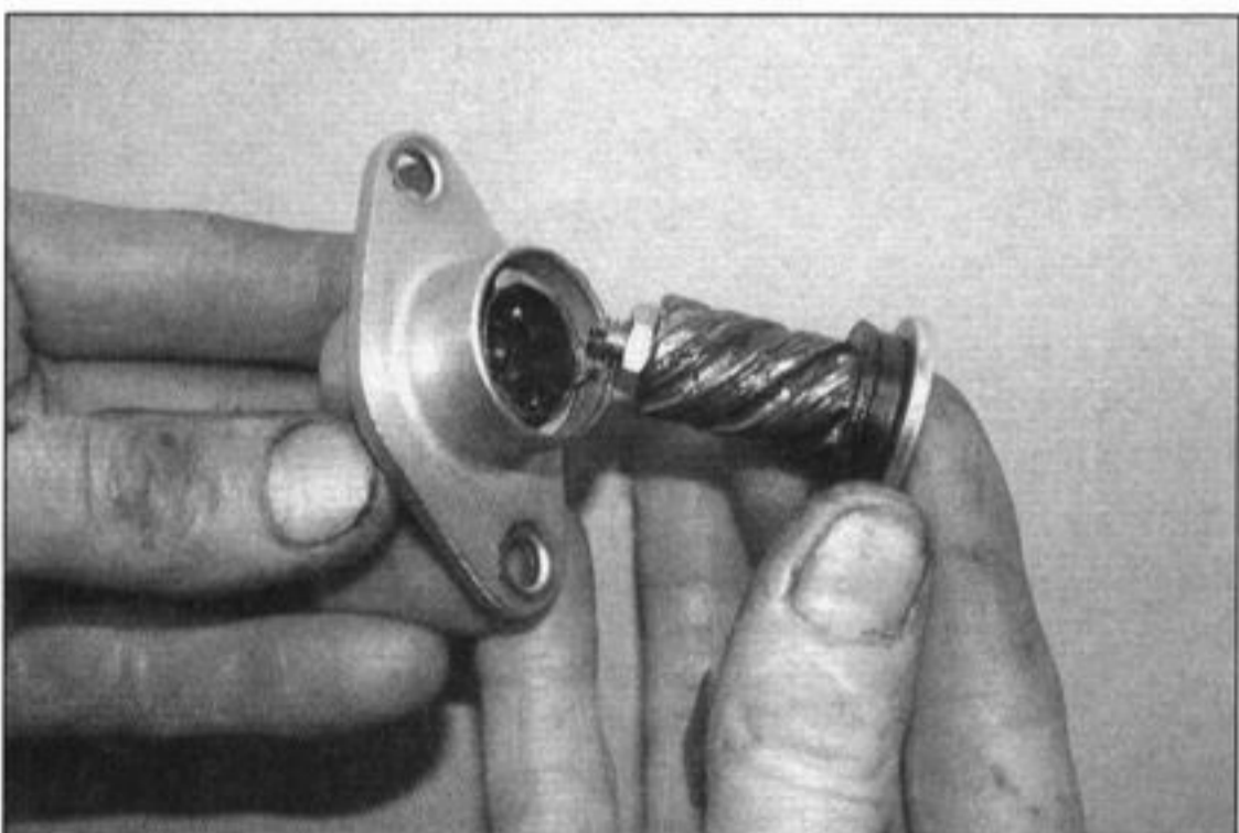
18.20c . . . then disassemble it, clean it and re-grease it
