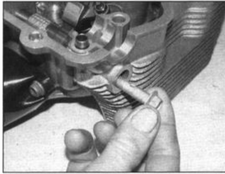
11.38 Thread an M8 bolt into the end of the rocker shaft and use it to withdraw the shaft
