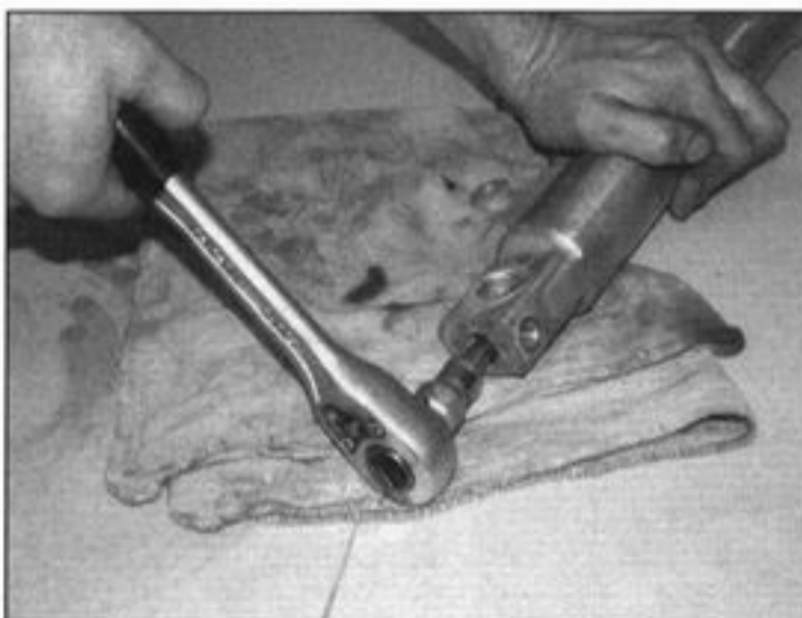
8.2b Slacken the damper rod bolt
