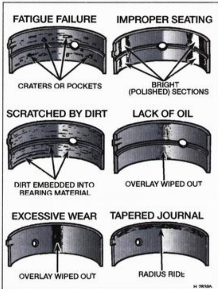
5.17 Typical bearing failures
