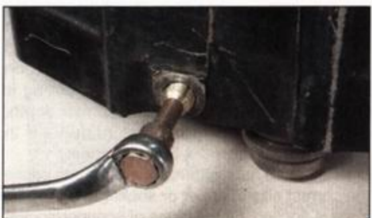
2.22 A thread repair tool being used to correct an internal thread
