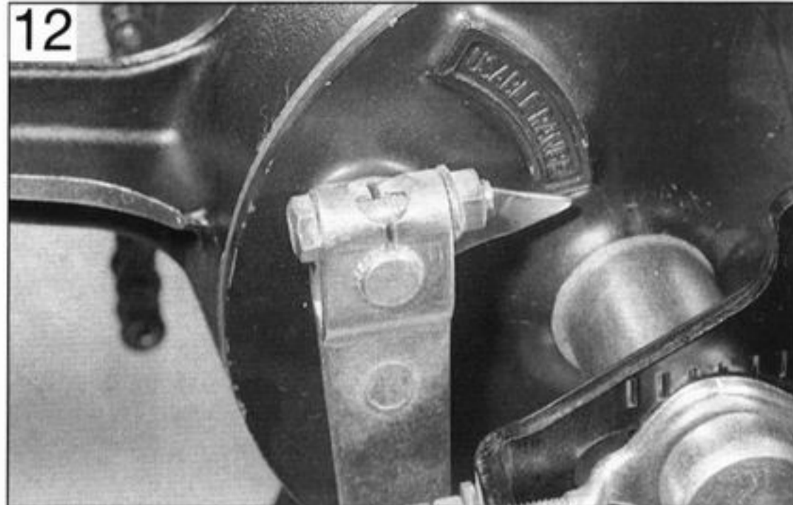
12 On drum brakes, check the angle of the operating lever with the brake fully applied. Most drum brakes have a wear indicator pointer and scale.
