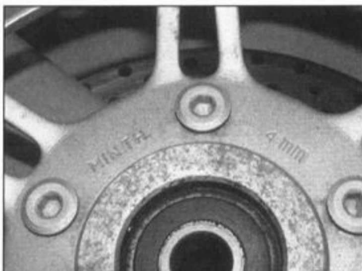
3.3a Front disc minimum thickness markings
