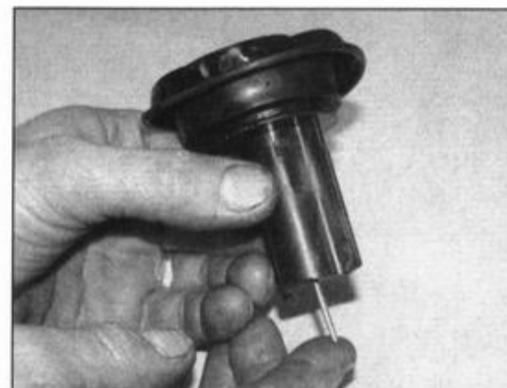
8.4b . . . then push the needle up from the bottom and withdraw it, noting the washer
