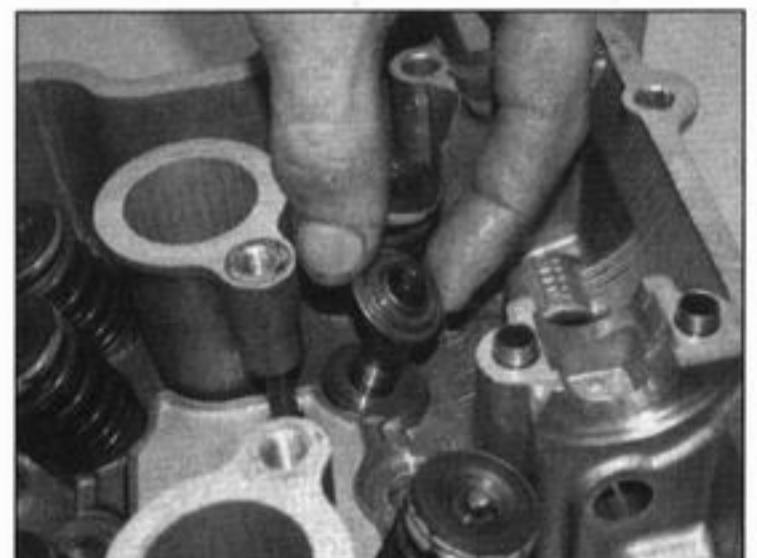
14.28 Fit the spring seat, making sure it is the correct way up
