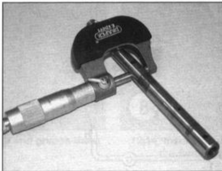
11.43a Measure the external diameter of the rocker arm shaft . . .
