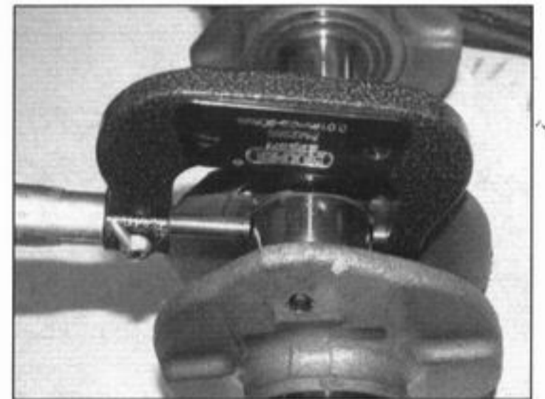
28.18 Measure the diameter of each crankpin journal
