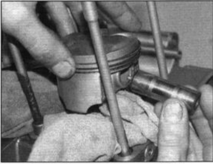
16.17a Line the piston up with the connecting rod and slide in the pin
