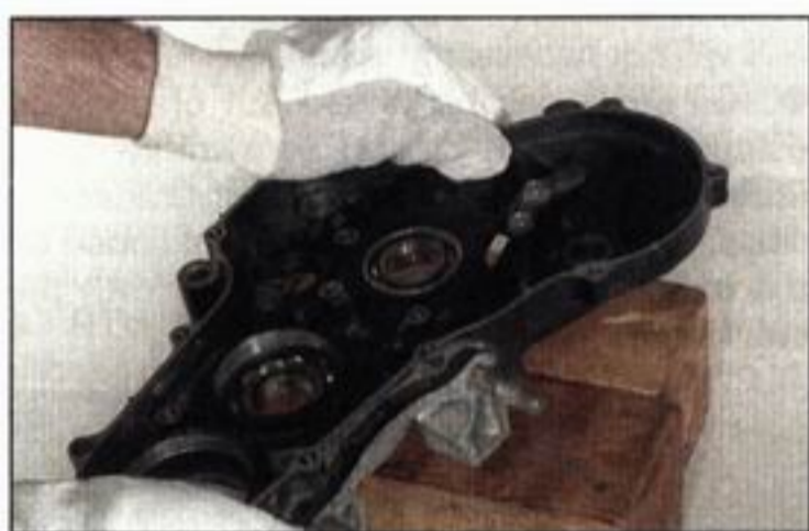
5.8 Tapping a casing face down on wood blocks can often dislodge a bearing
