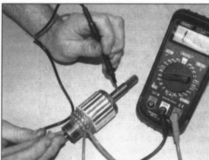
30.8b There should be no continuity between the bars and the shaft
