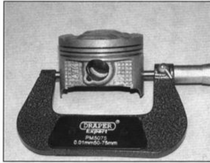
16.11 Measure the piston diameter at the specified distance from the bottom of the skirt
