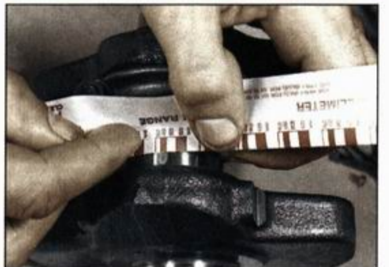
3.16 Measuring the width of the crushed Plastigauge
