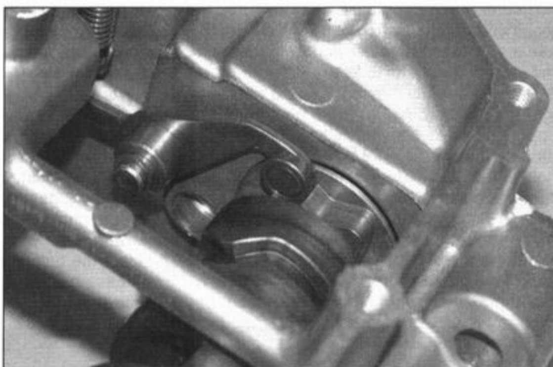
29.29 Locate the roller in the neutral detent in the cam
