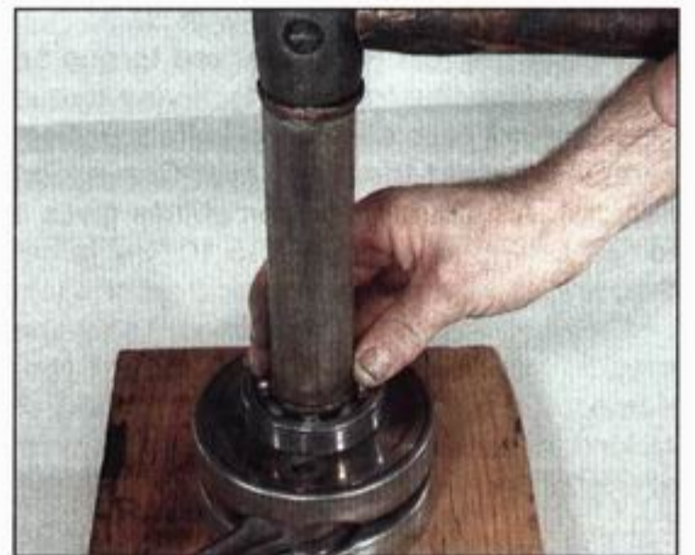
5.5 When installing a bearing on a shaft use a piece of tubing which bears only on the bearing's inner race
