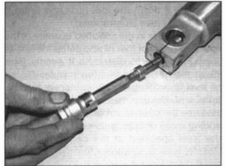
8.19b . . . then fit the bolt using threadlock and a new sealing washer . . .
