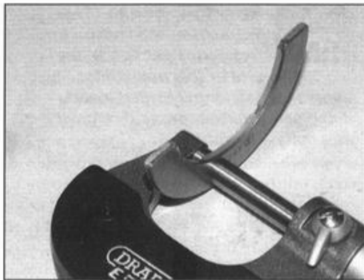
27.10 Measure the thickness of the right-hand (inner) thrust bearing
