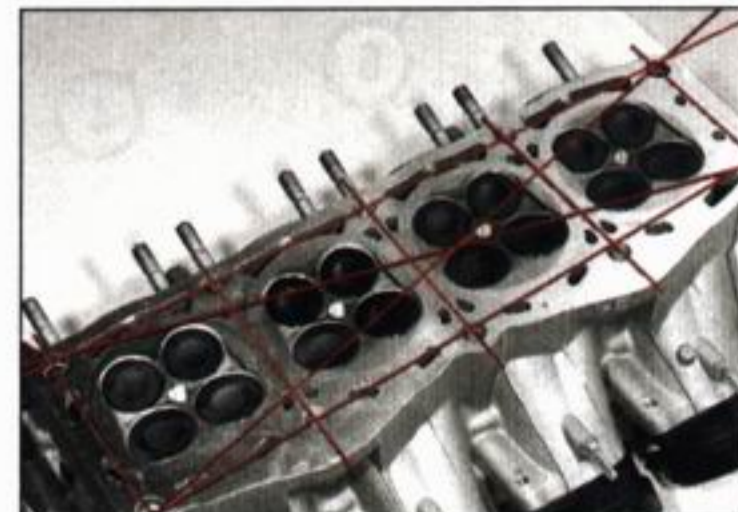
3.23 Check for warpage in these directions
