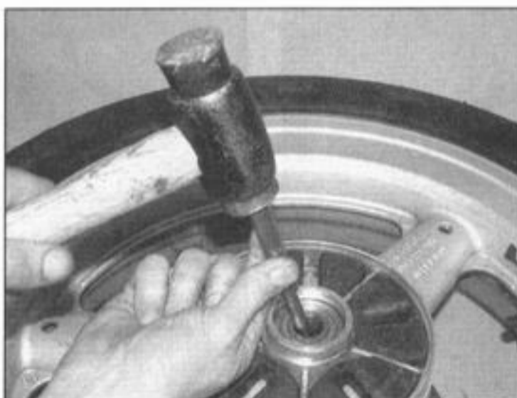
14.13 Drive the bearings out as described
