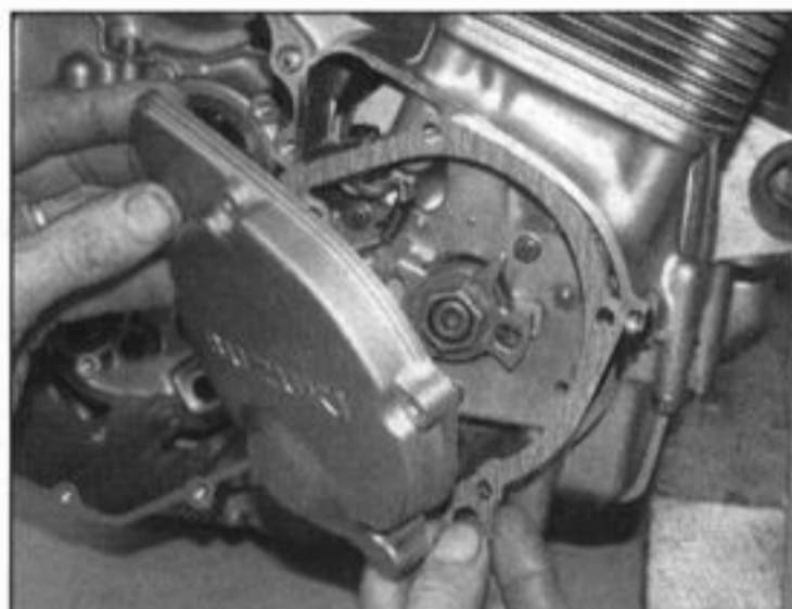
11.35b Fit the cover using a new gasket . . .
