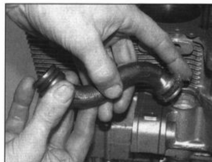
15.28 Use a new O-ring on each oil drain tube and smear them with grease
