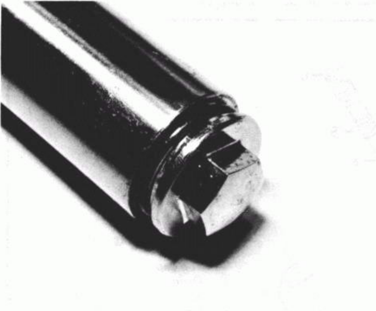
4.13d ...and loosely refitting the cap bolt and O-ring to prevent rotation of the damper rod
