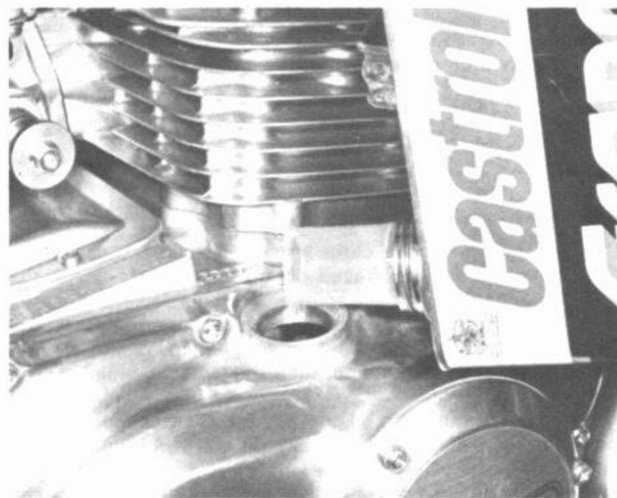
If required, replenish the oil reservoir with SAE 10W/40 engine oil
