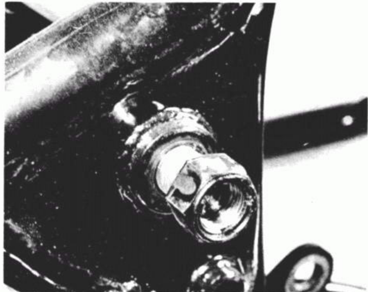
9.11g ...and securing it with the pivot shaft, plain washer and nut
