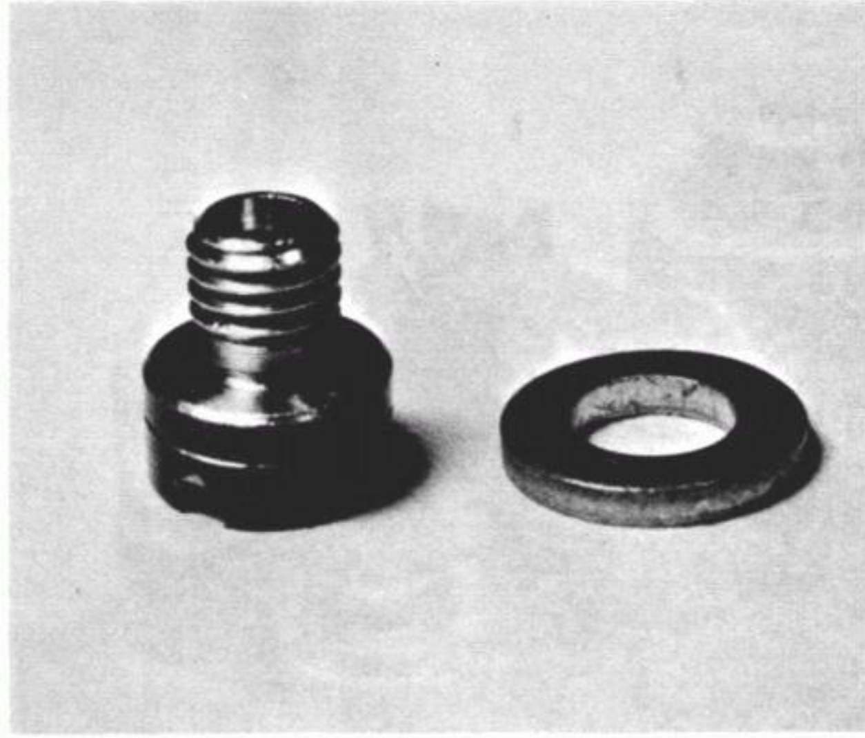
6.22c Fit the washer beneath the head of the main jet...
