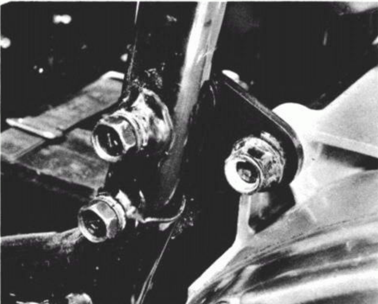
4.23b ...and finally, the upper rear mounting plate...
