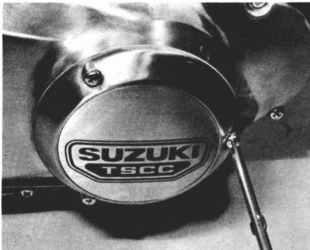
7.2 The ignition timing assembly is located beneath its circular cover
