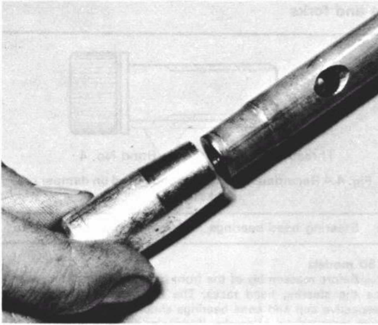
4.13b ...refitting the damper rod seat...
