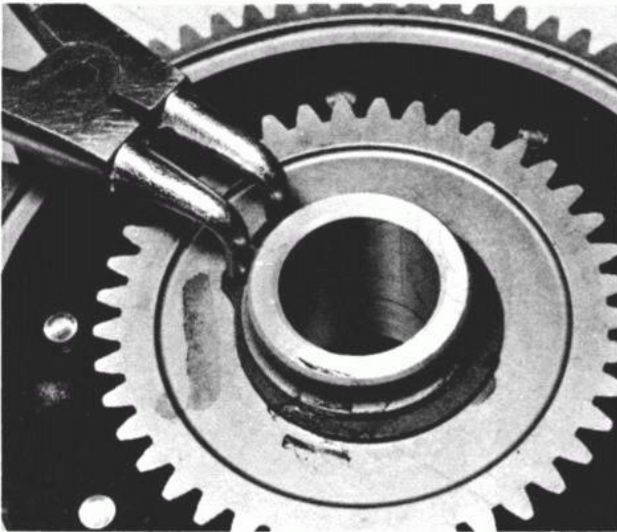
38.2c ...before securing the pinion with the circlip
