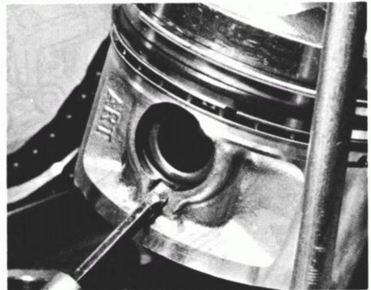
7.7 Prise each gudgeon pin circlip from position
