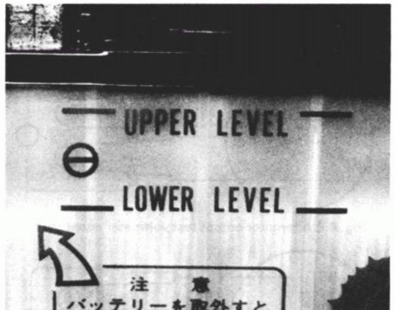
7.1 The battery electrolyte should be kept between the two level marks
