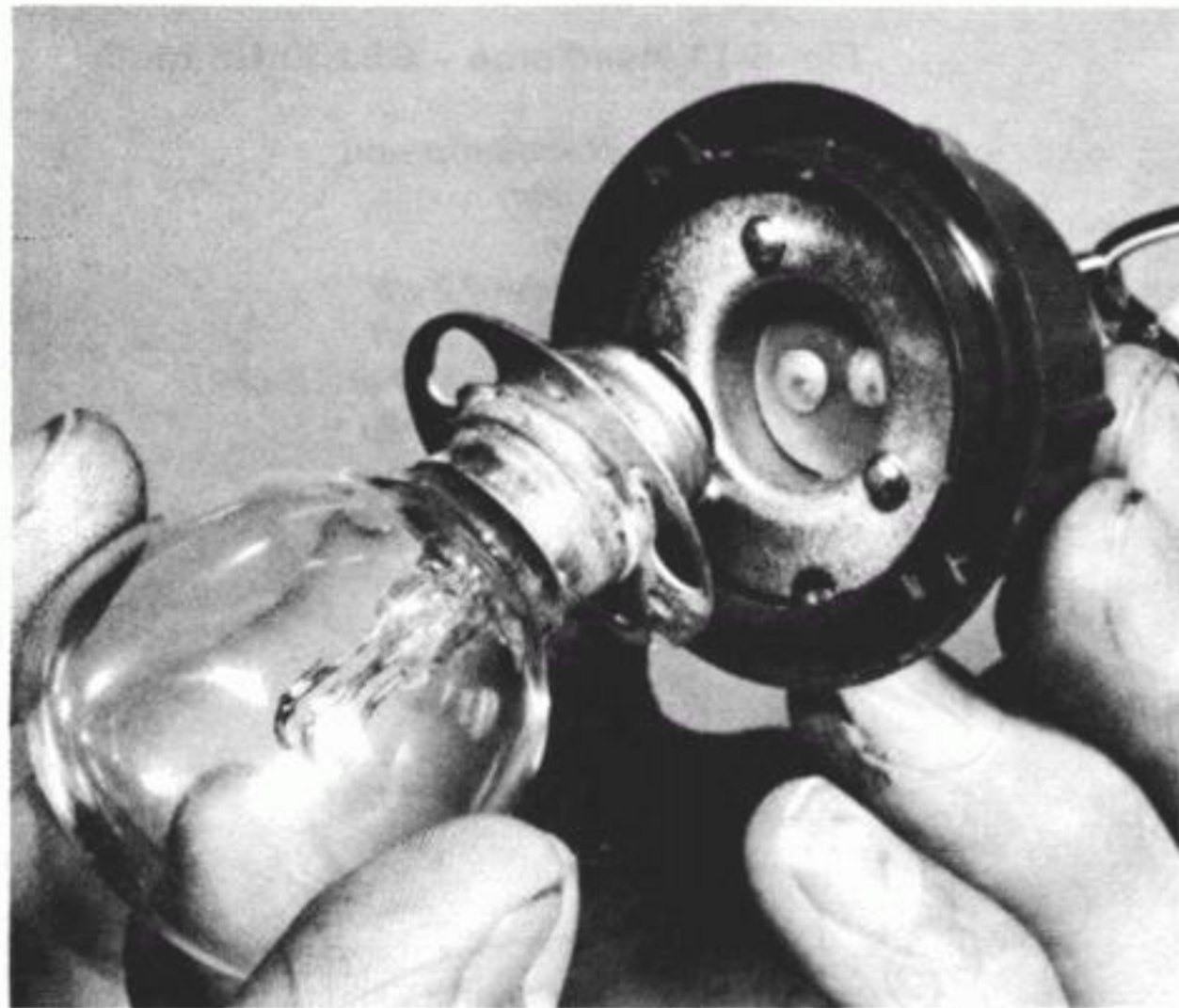
31.2b ...to allow removal of the main headlamp bulb
