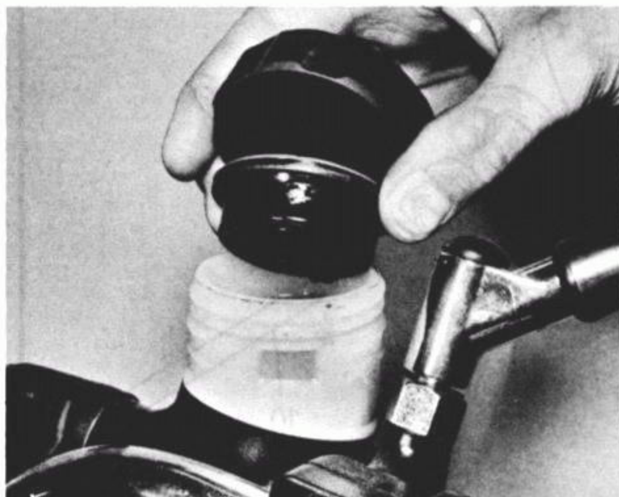
5.2 Remove the reservoir cap and diaphragm assembly
