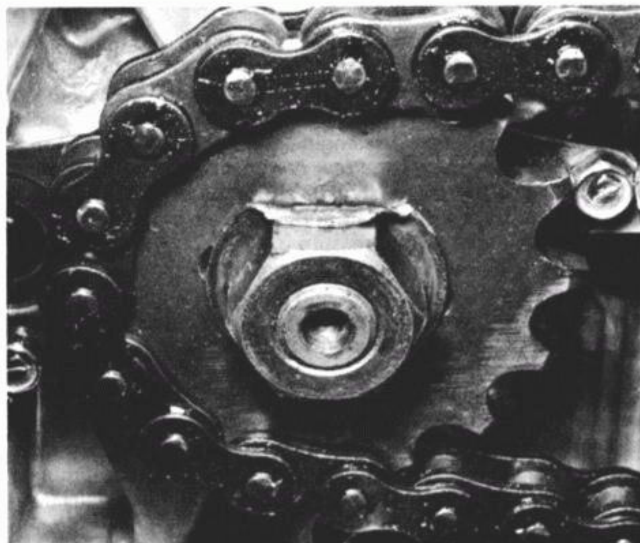
46.3b ...before fitting the nut and locking it in position with the tab washer
