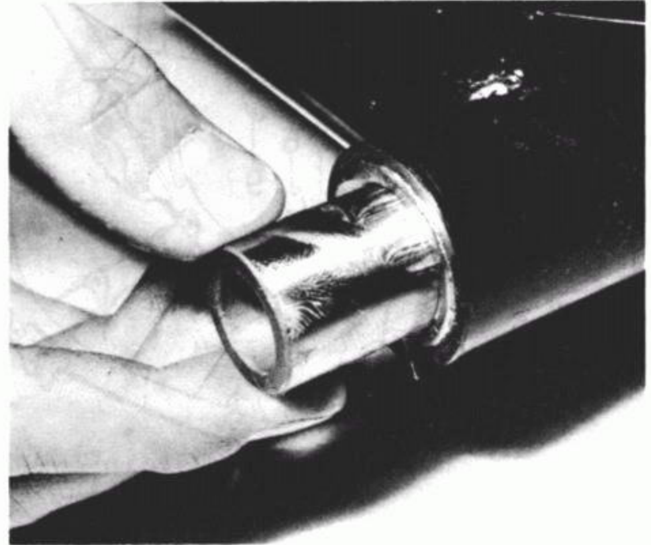
9.11c ...before inserting each bush into position
