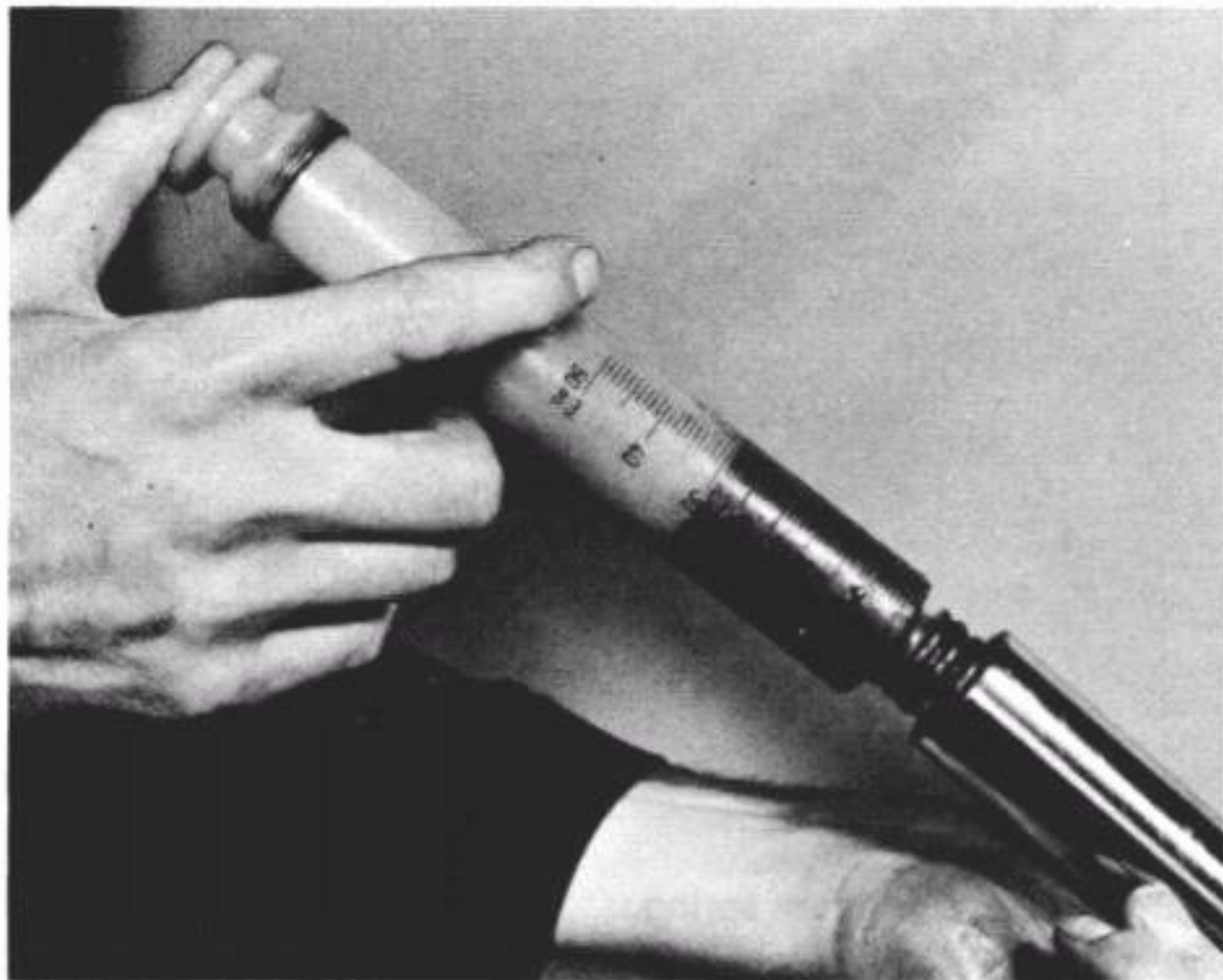
4.14b Remove the cap bolt to allow replenishment of the fork leg oil
