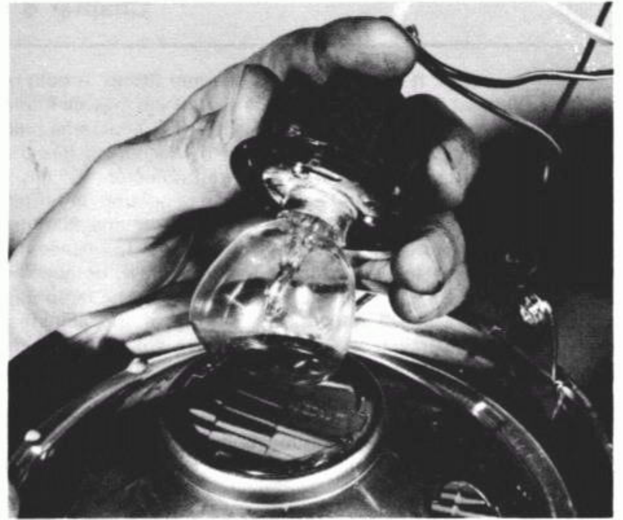
31.2a Detach the bulb holder from the reflector...
