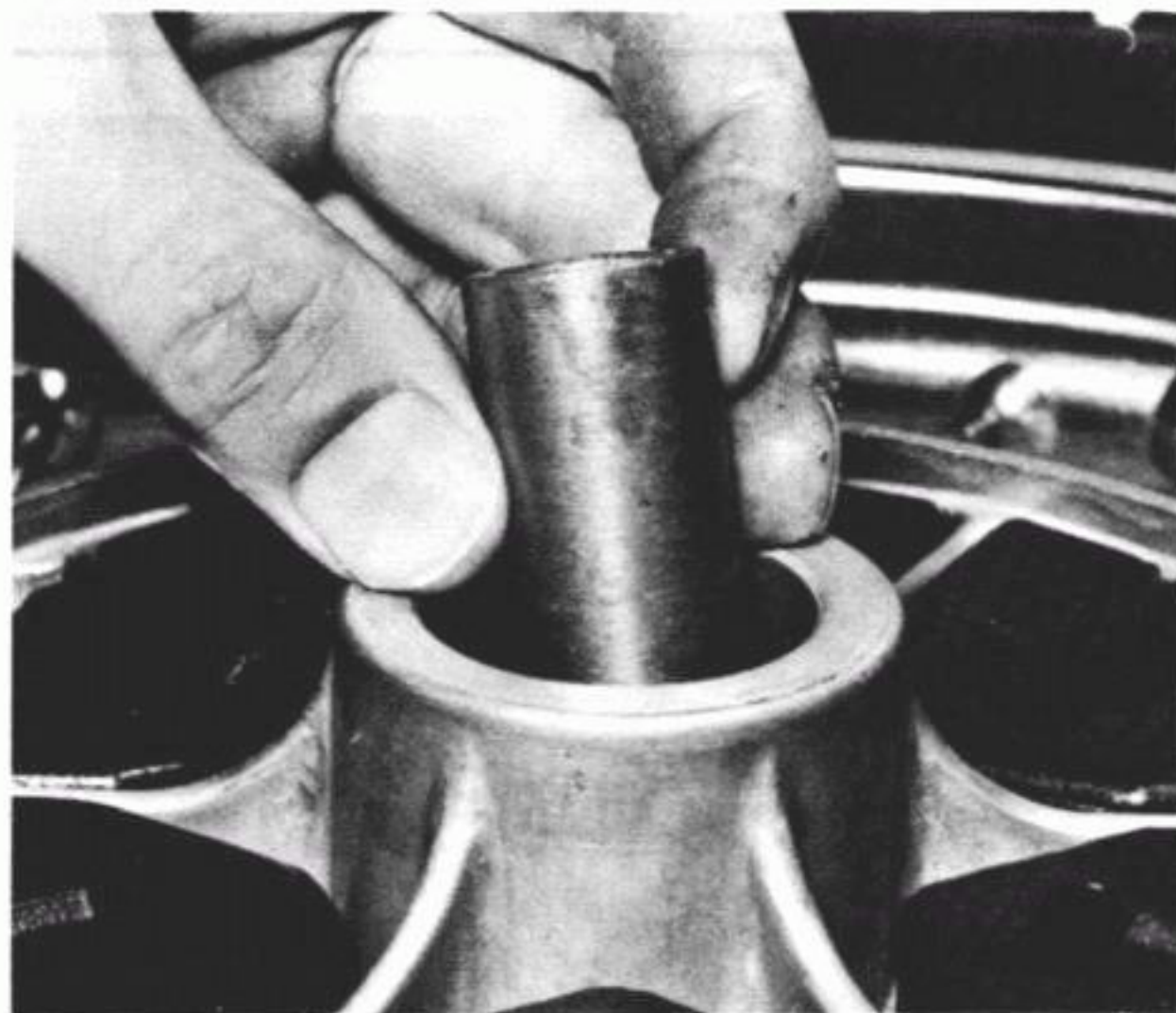
12.5b ...grease and insert the bearing spacer...
