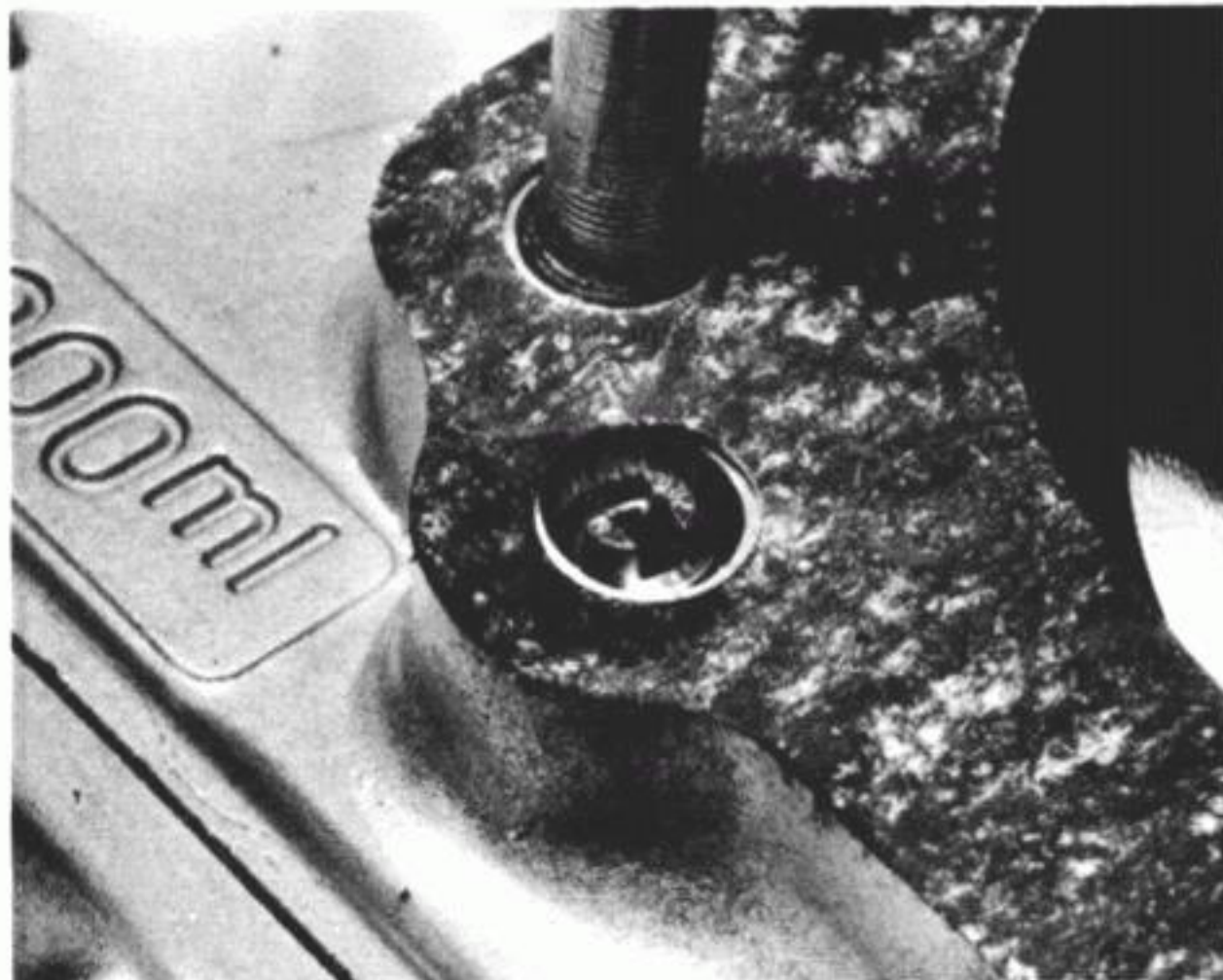
7.5 ...and the oil supply jets located on the edge of each crankcase mouth
