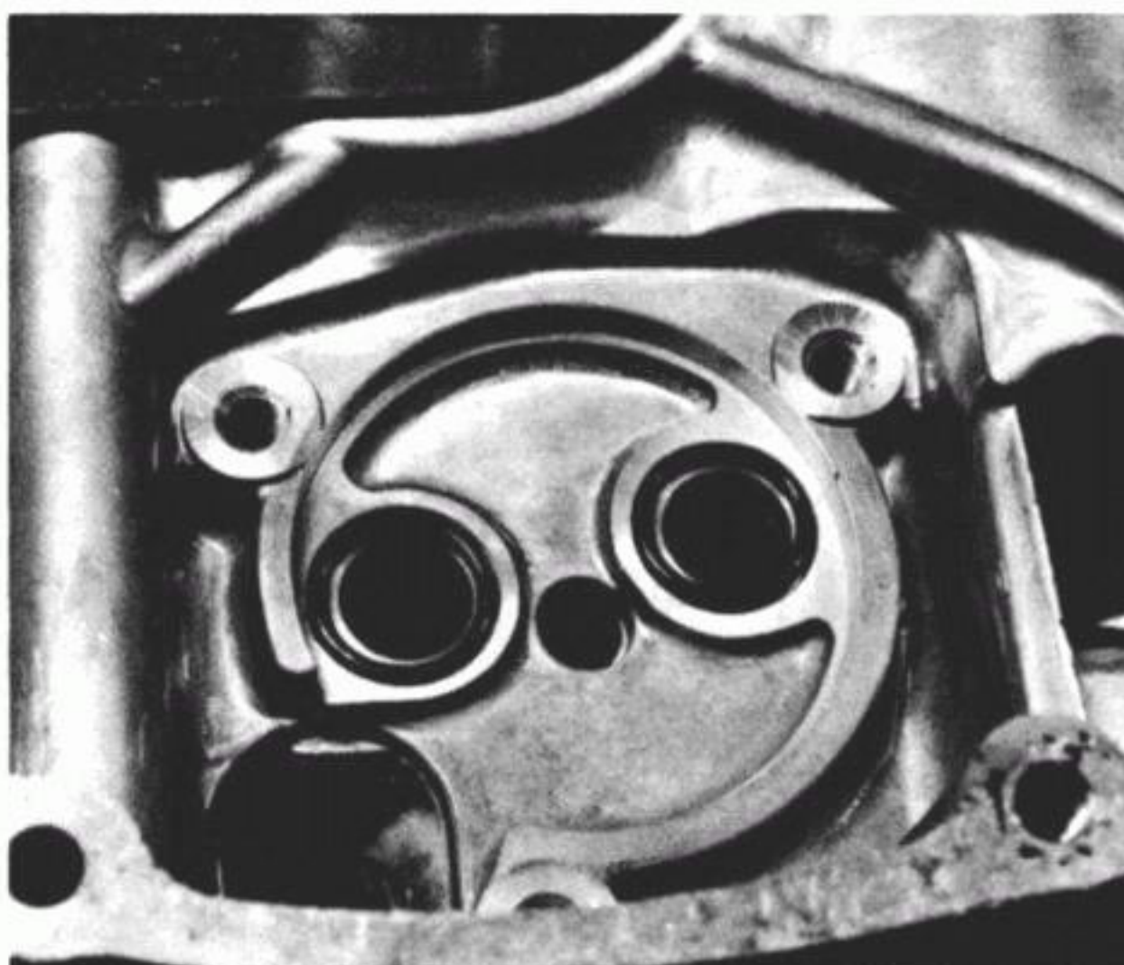
14.9b Lubricate and fit new O-rings into the crankcase...
