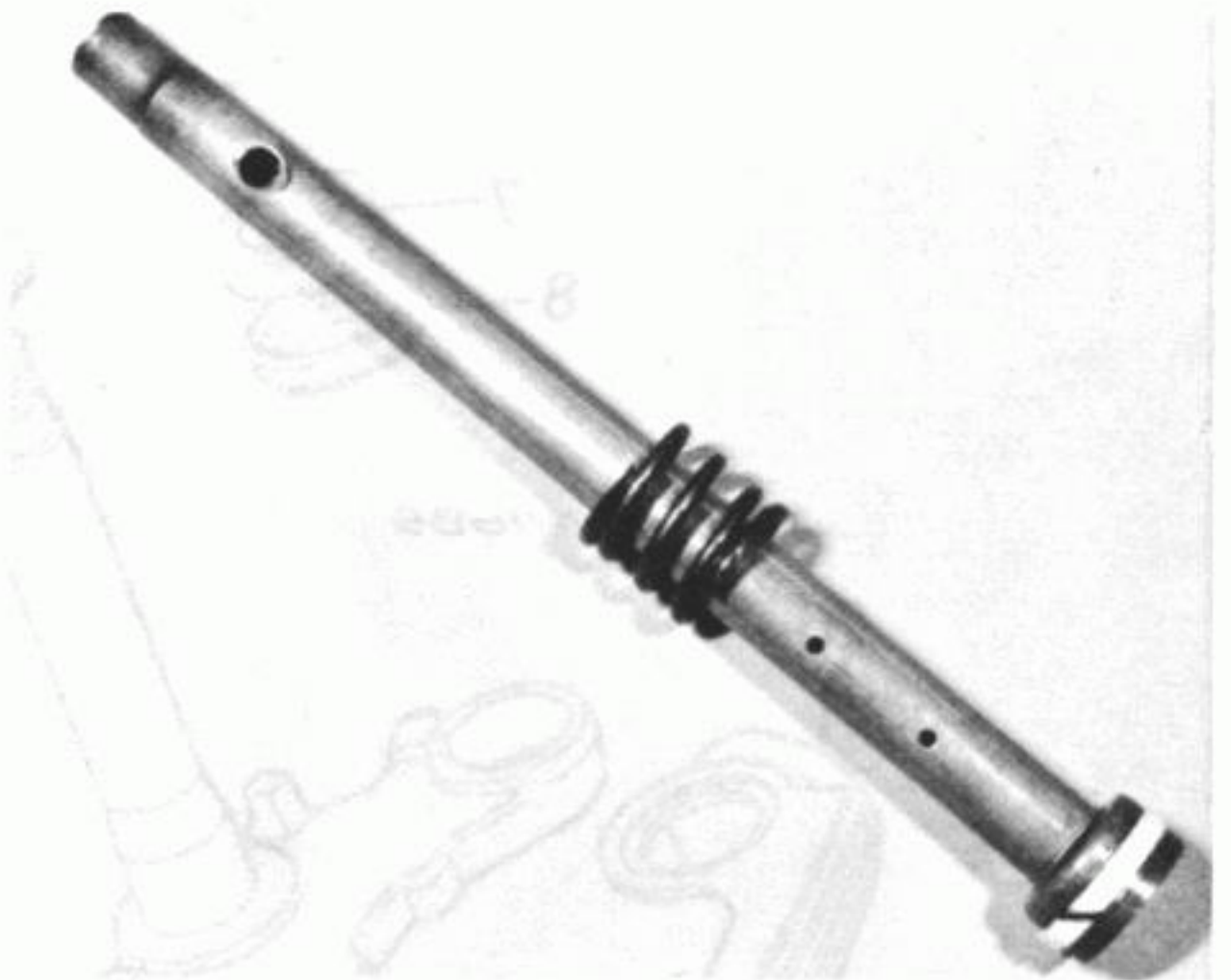
4.8 Inspect the damper rod assembly for ring and spring wear
