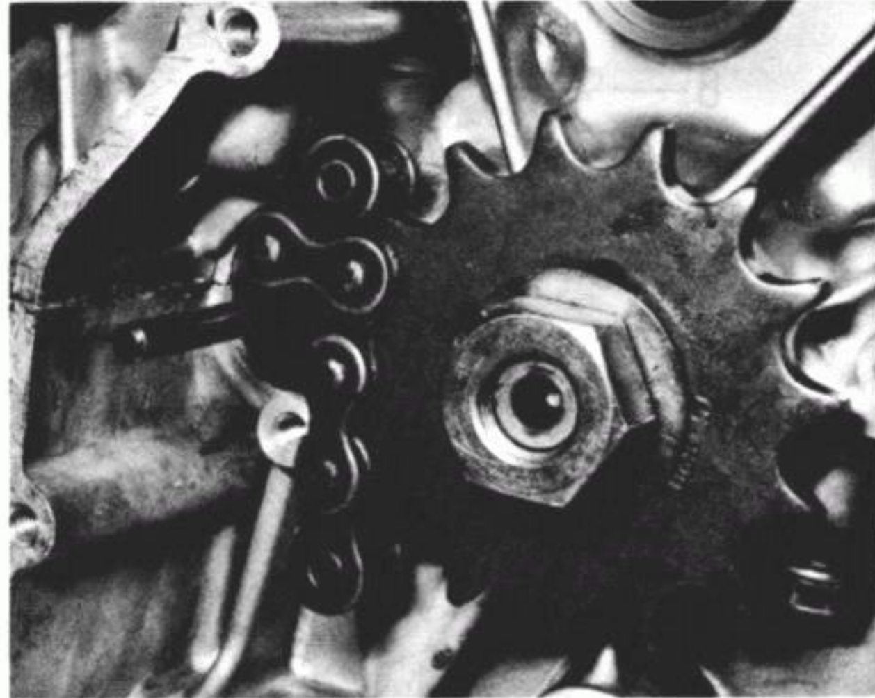
10.3 Use a short length of final drive chain to lock the gearbox sprocket in position
