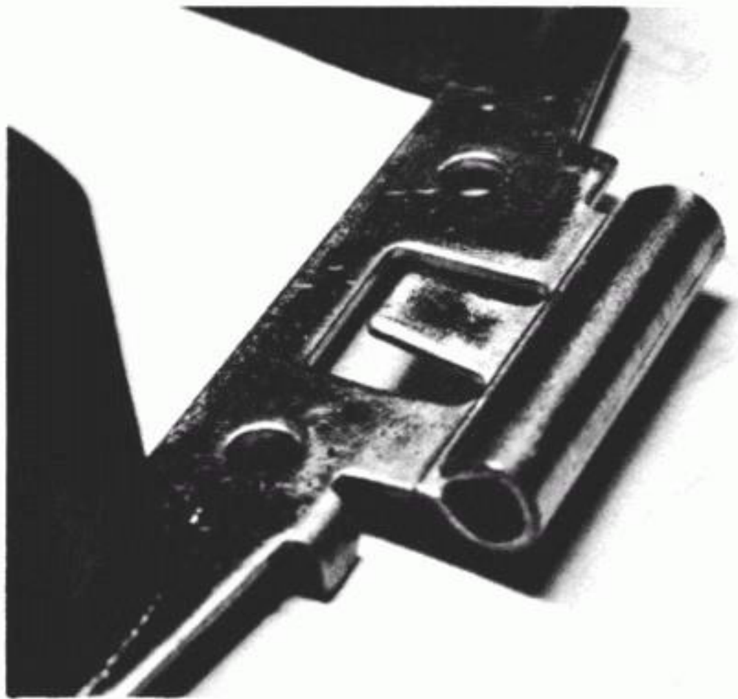
8.6 Bend the float pivot tang to adjust the float height
