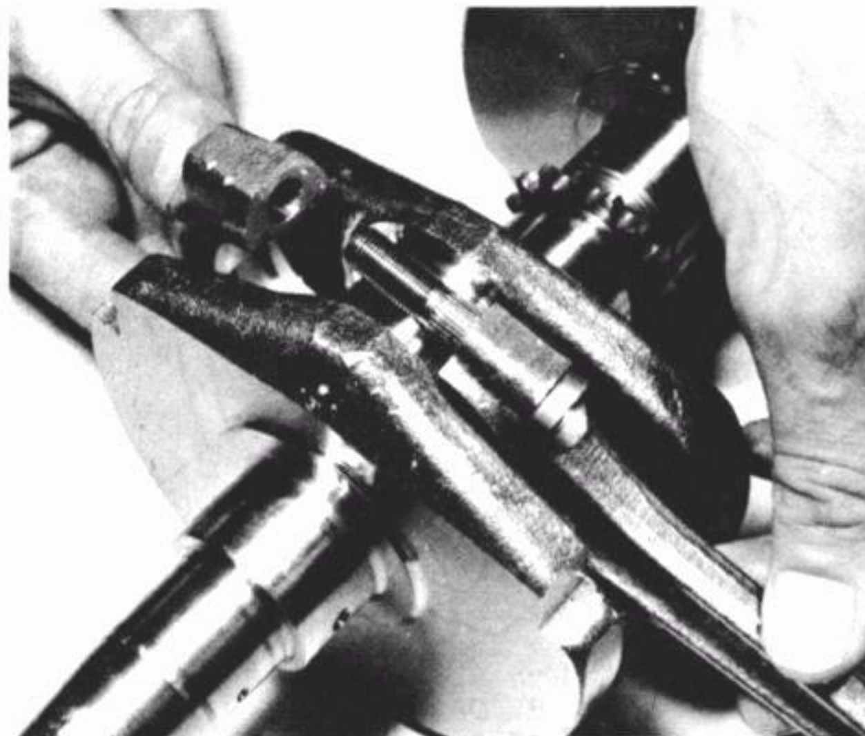
17.9a ...fit the connecting rod to the crankshaft...
