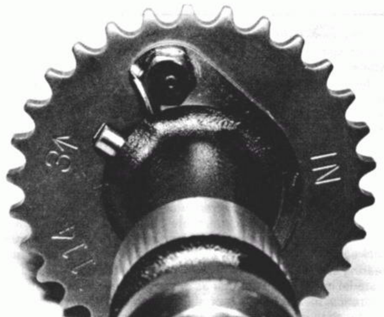
24.4 Note the camshaft sprocket markings, the locating pin and the lock washer
