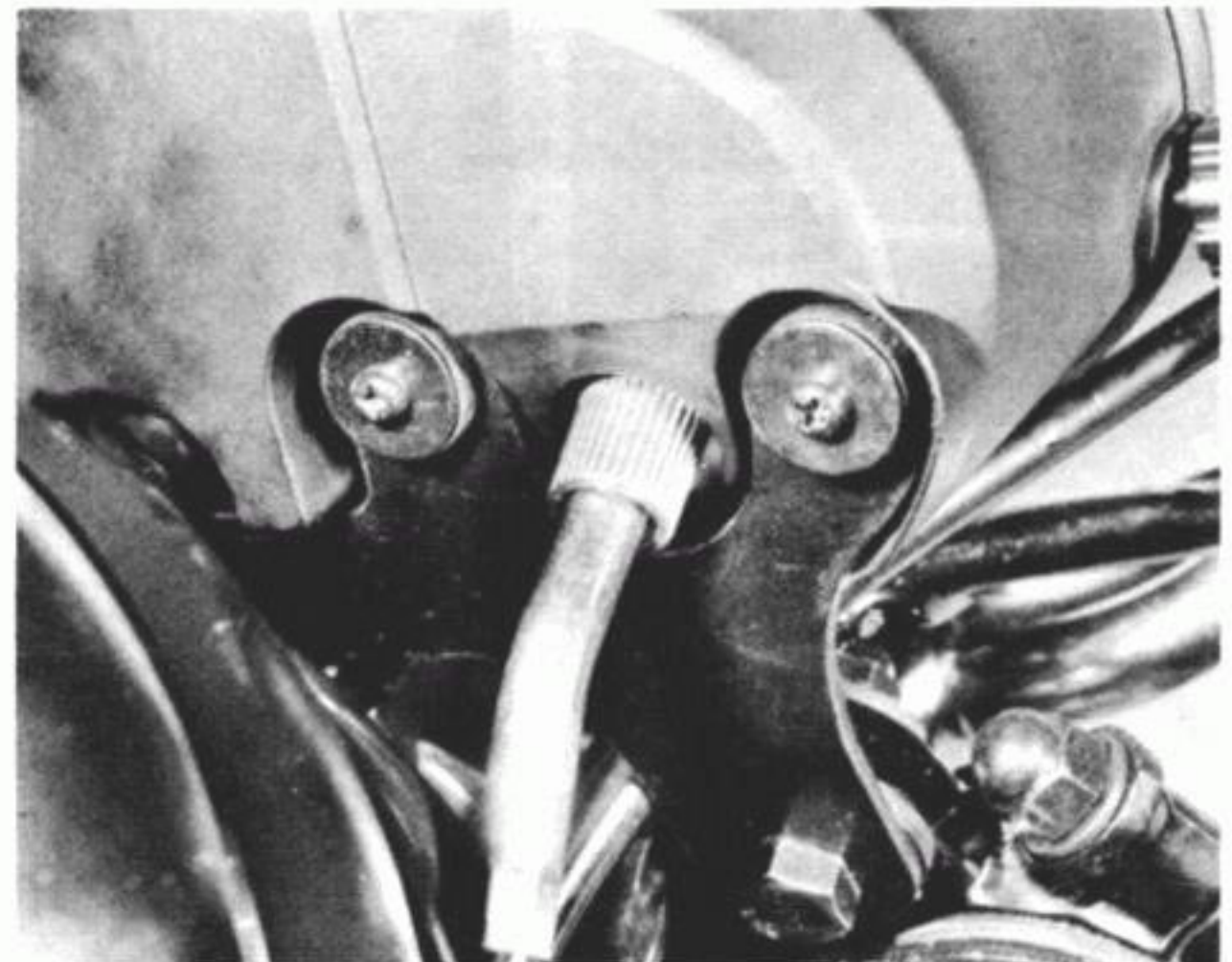
16.1 Each instrument head is secured by two crosshead screws
