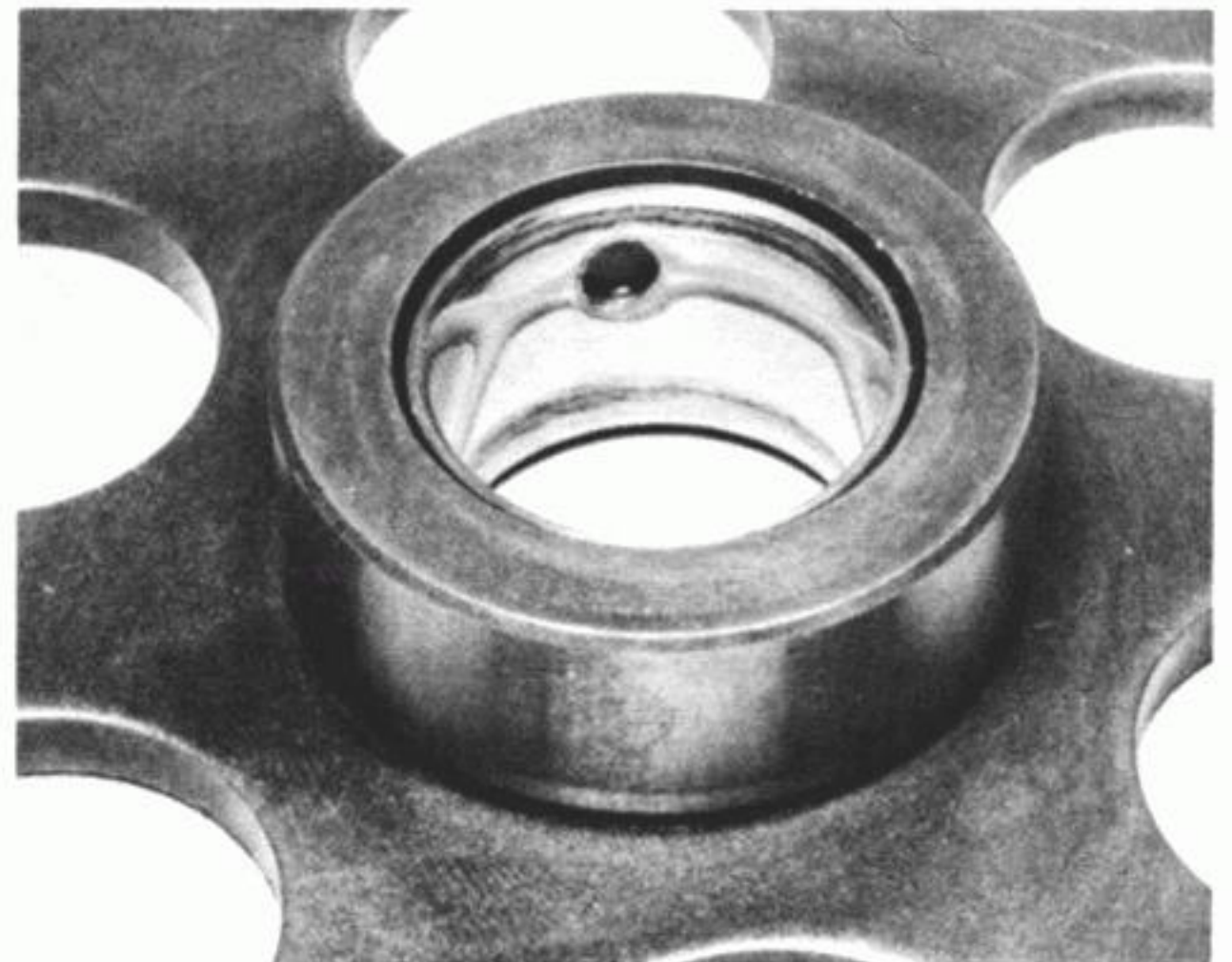
11.6 Inspect the starter clutch sprocket boss and bush for wear or damage
