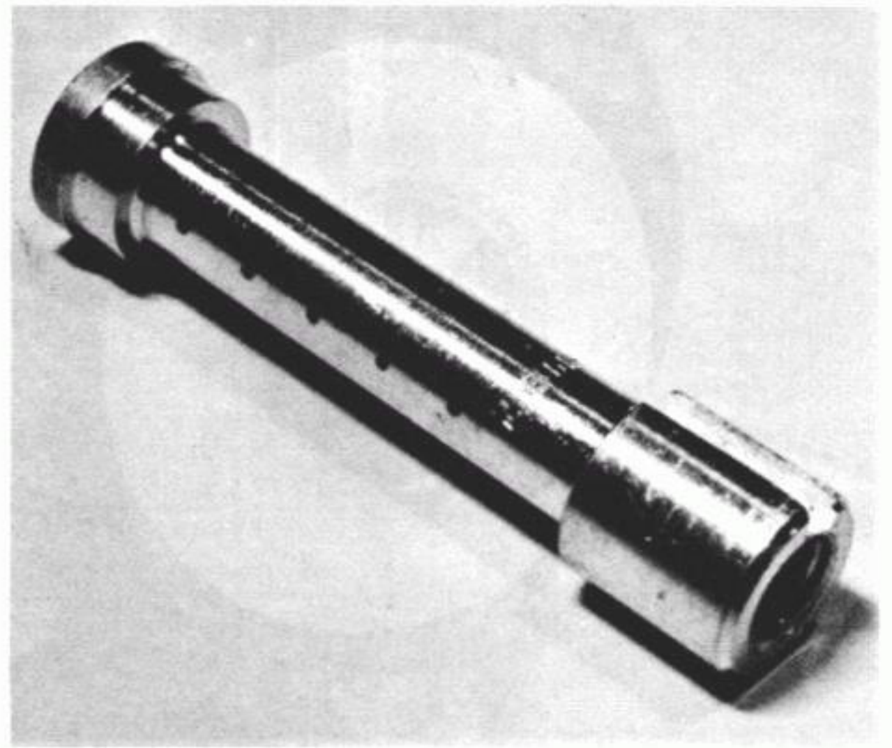
6.15b ...and blow clear any blocked jets with compressed air (needle jet shown)
