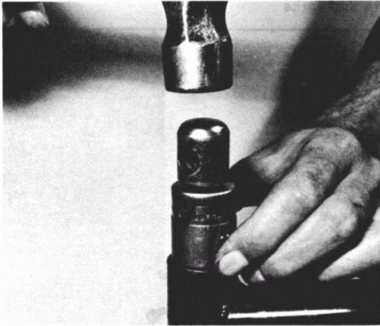
9.8c ...and a length of thick-walled metal tube to drift new bearings into position
