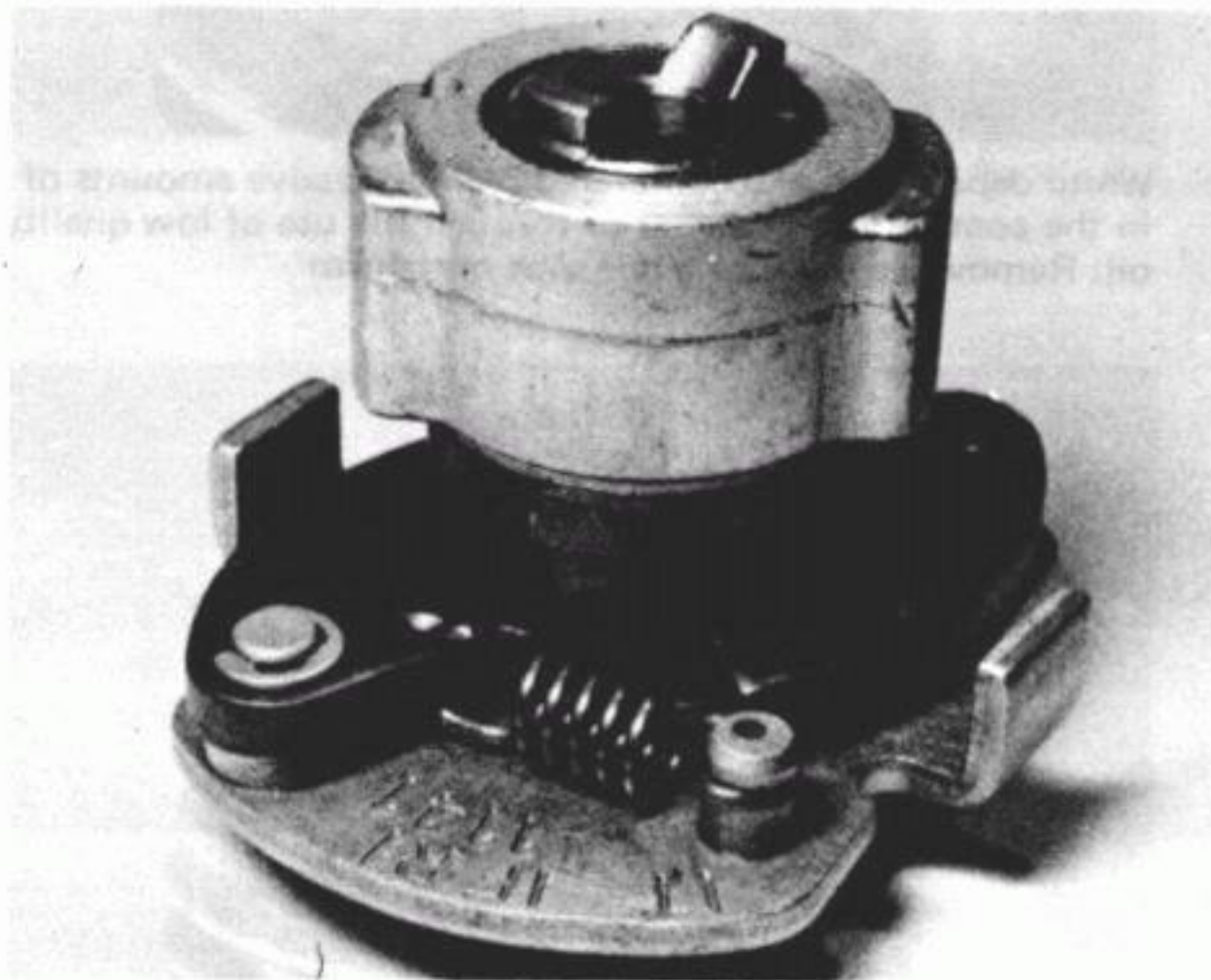
8.2 Inspect the ATU spring and pivot assemblies
