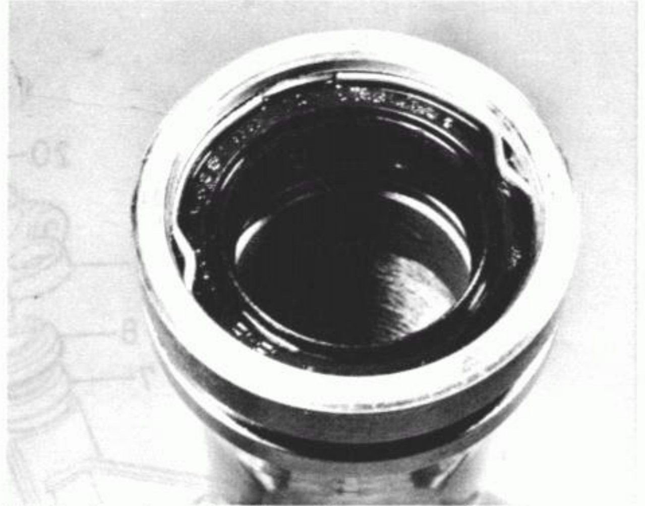
4.4 Displace the spring clip to allow removal of the fork leg seal
