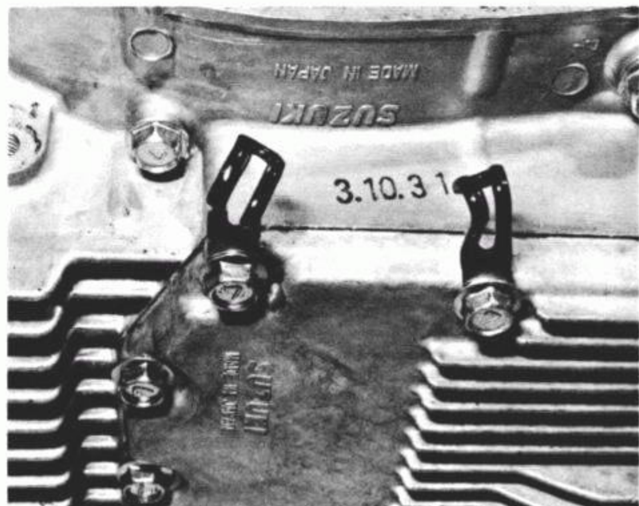
36.8b Correctly position the two electrical cable retaining clips beneath the bolt heads
