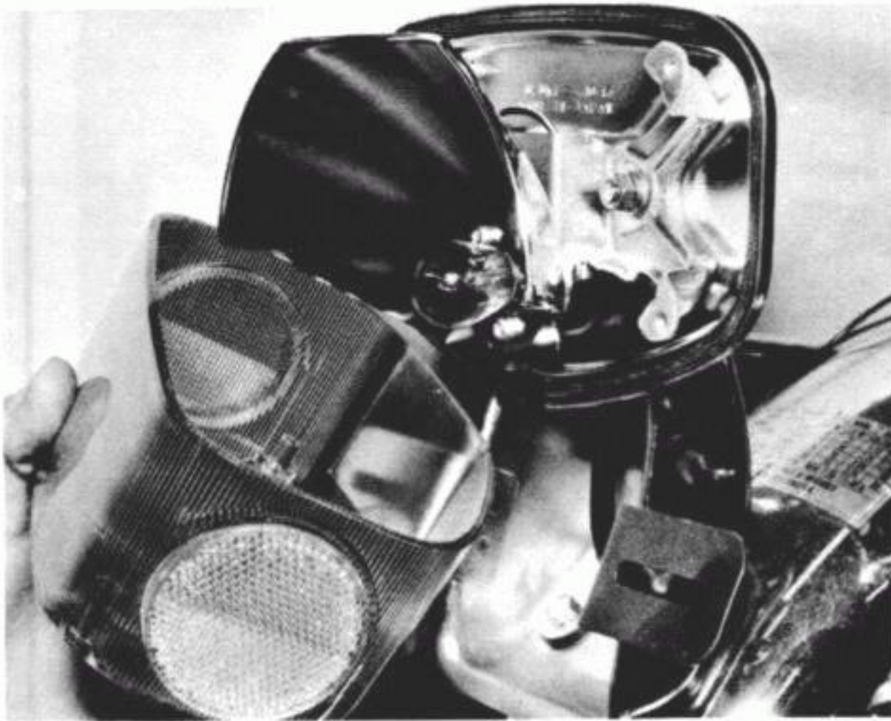
32.3 Remove the plastic lens cover to gain access to the tail lamp bulb
