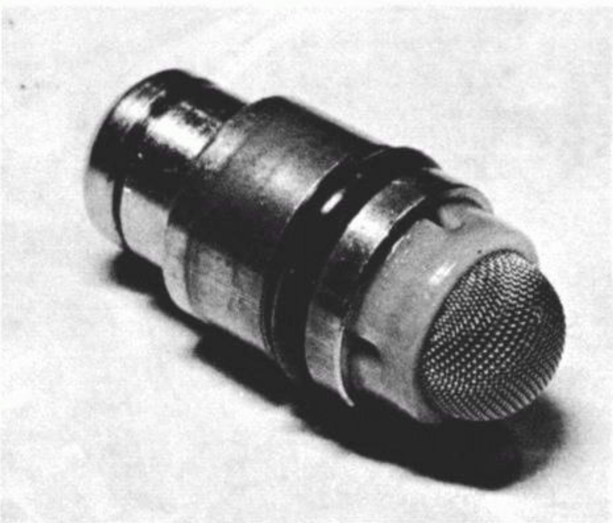
6.12b ...whilst checking that the filter attached to the seating is clean
