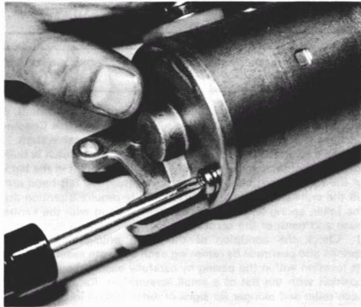
10.10c ...before tightening the assembly cap securing screws
