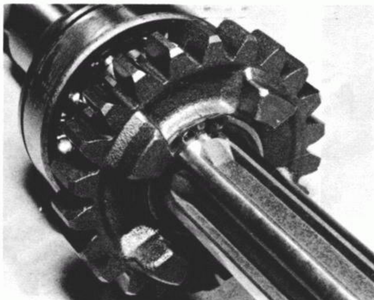
28.8c ...and retaining it in position with the washer and circlip
