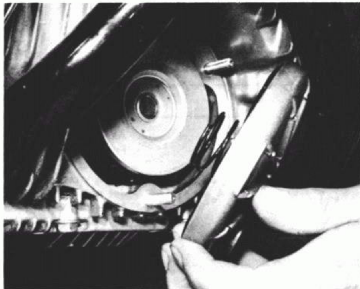
16.3 A coil spring is fitted between the filter element and cover
