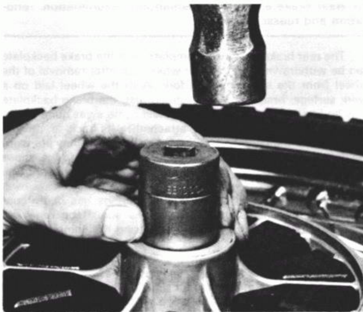
12.5d Drift the left-hand bearing into position...
