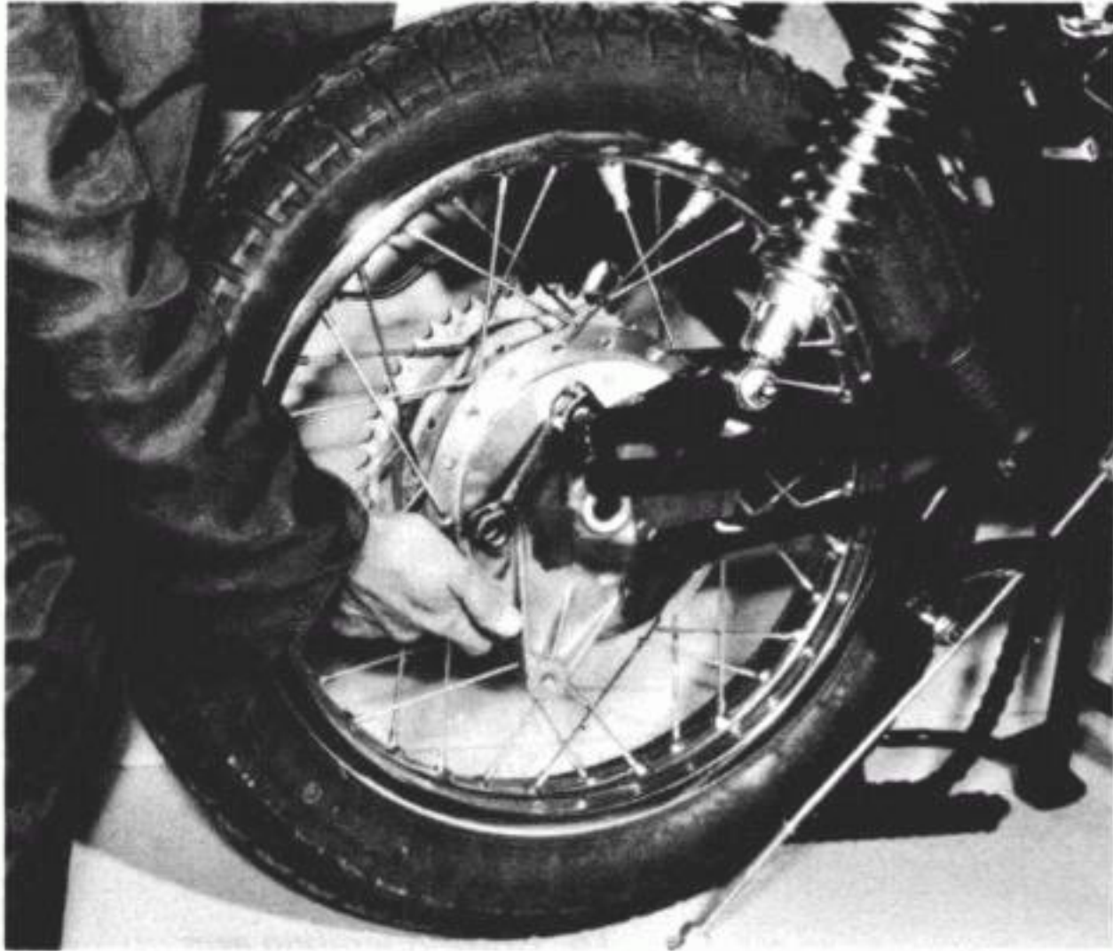
11.6a Lift the rear wheel assembly into the swinging arm fork
