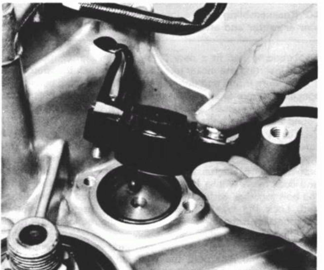
40.6 Do not omit to fit the neutral indicator (or gear position) switch contact pin and spring and a new O-ring
