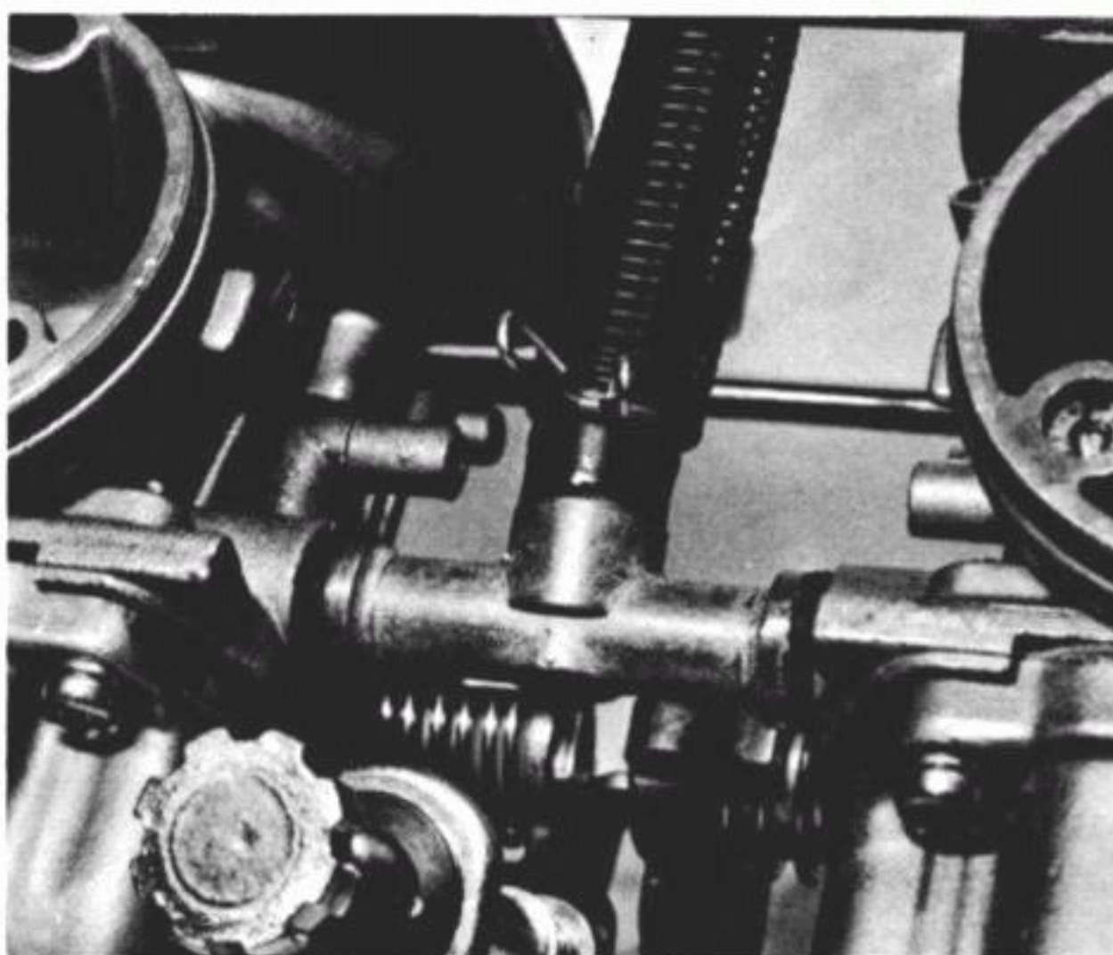
6.18b The fuel cross-over pipe must be correctly located
