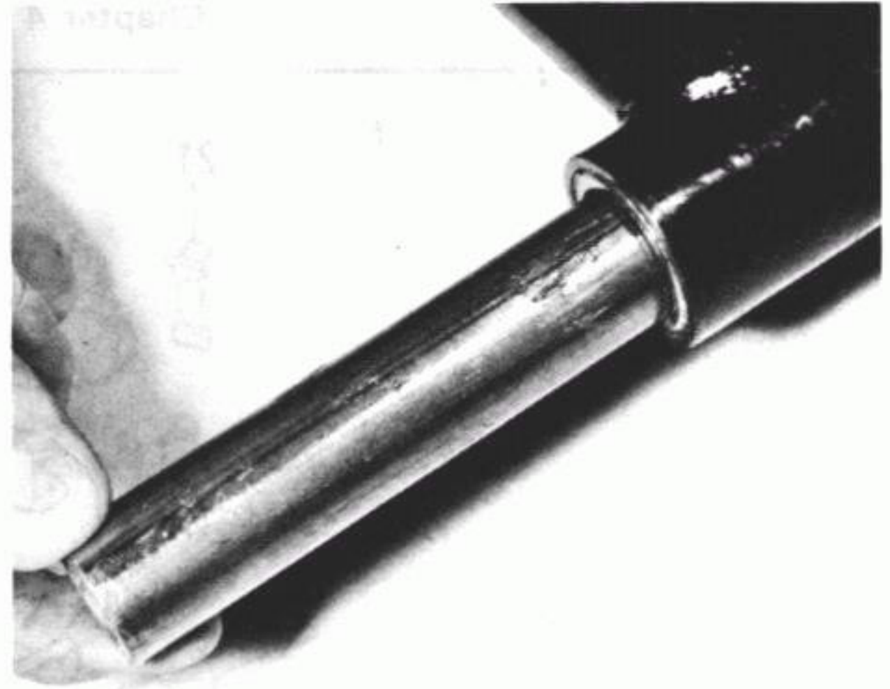
9.11a Commence reassembly of the swinging arm by greasing and inserting the central spacer
