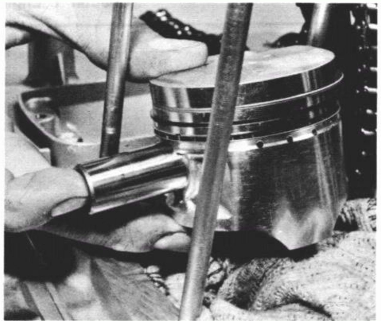
41.5b Lubricate the gudgeon pin before fitting
