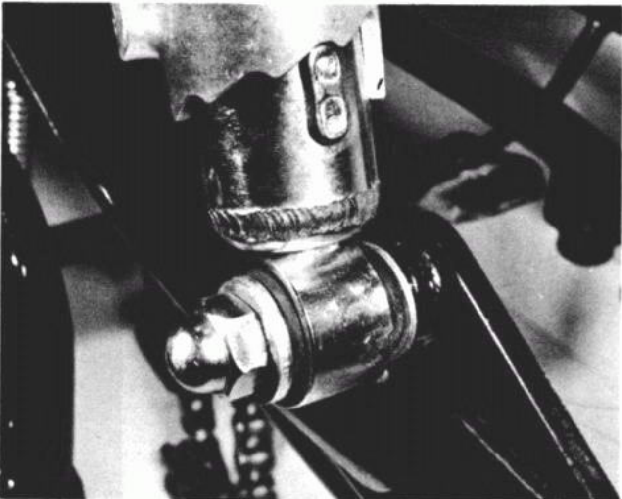
9.11h The rear suspension unit retaining nuts should be tightened to the correct torque loading
