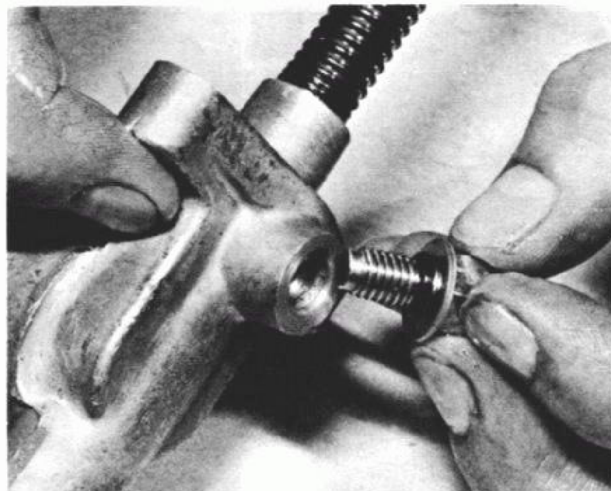
25.4f Renew the O-ring and gasket washer beneath the pushrod locknut
