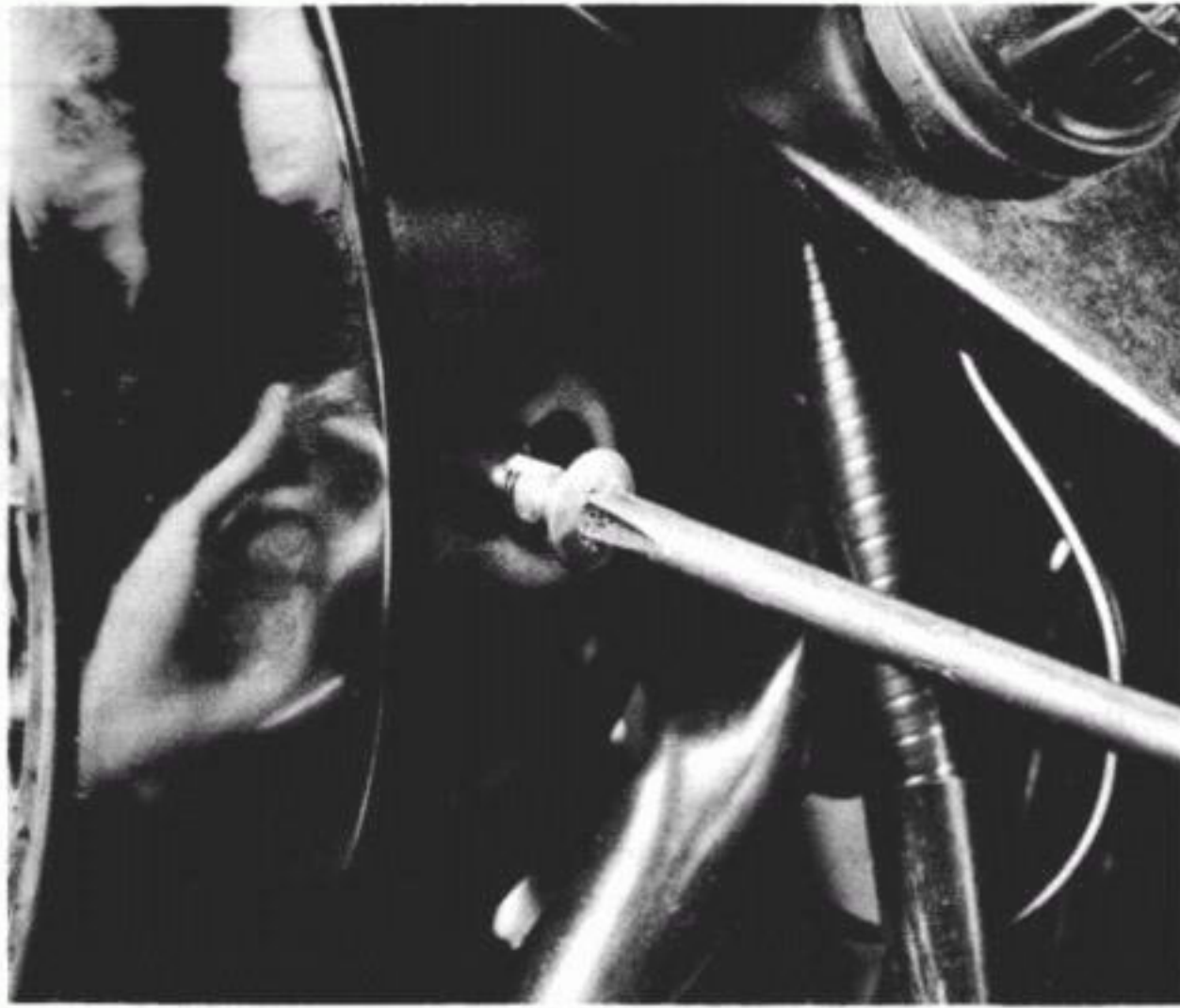
31.1 The headlamp rim is retained by three crosshead screws
