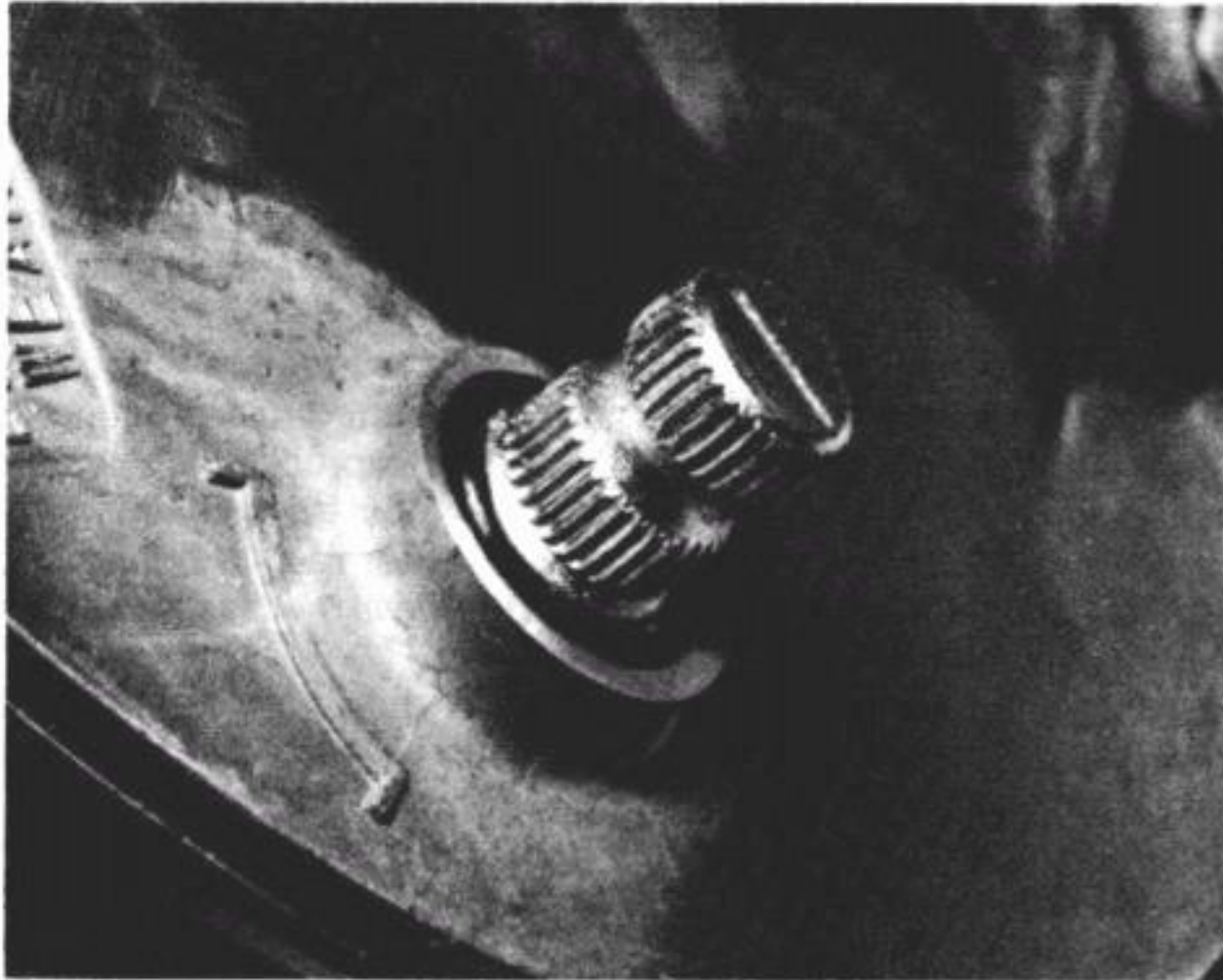
13.10a Fit a serviceable O-ring over the shaft...
