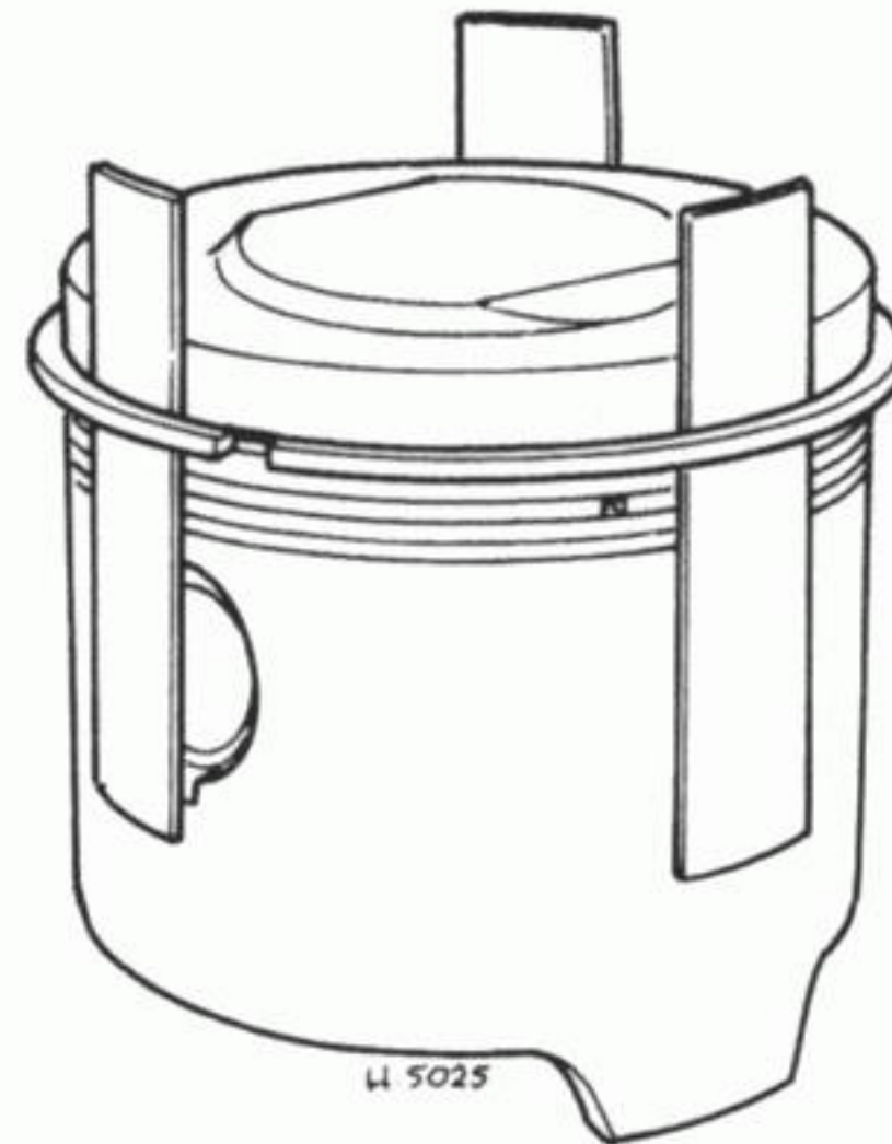
Fig. 1.10 Method of removing and replacing piston rings
