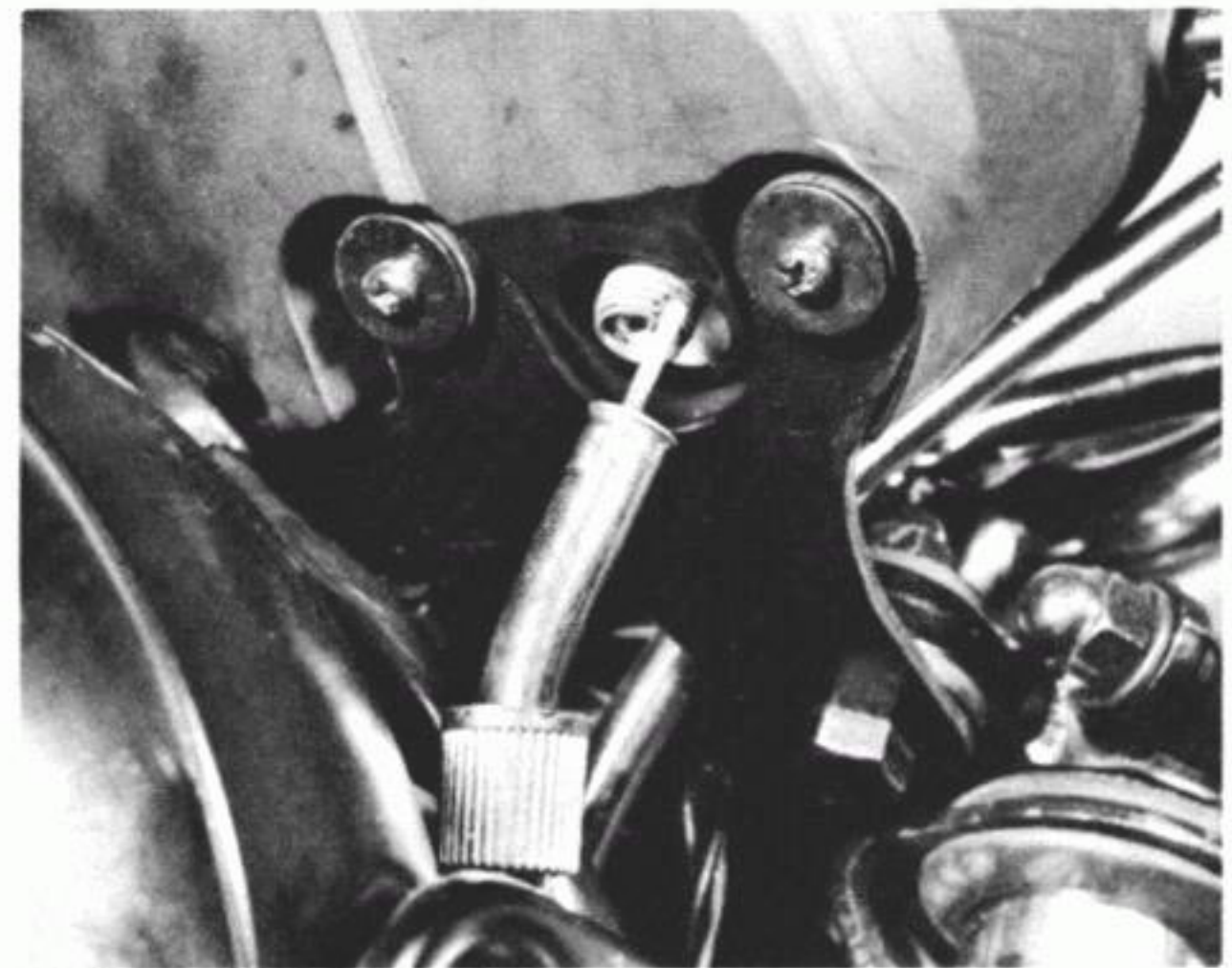
27.2 Detach each instrument head by removing its two retaining screws
