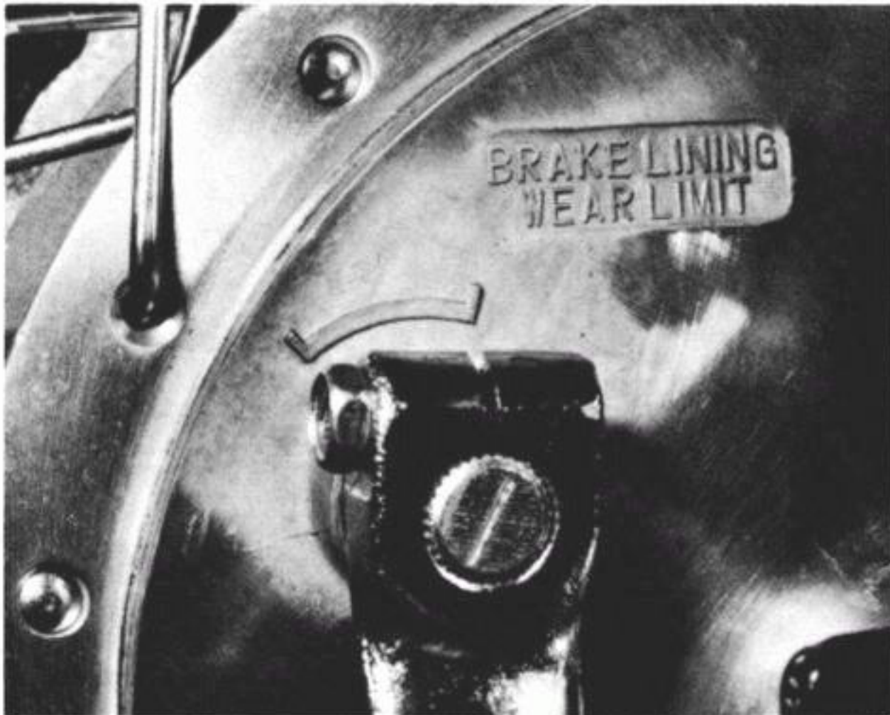
14.4 An indication of brake lining wear is provided
