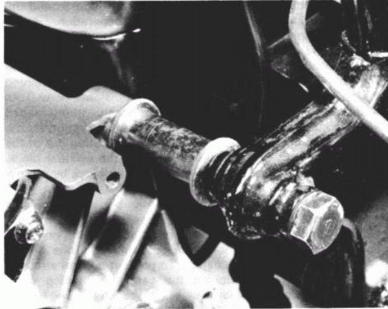
4.23c ...taking note of the cylindrical spacer and washers
