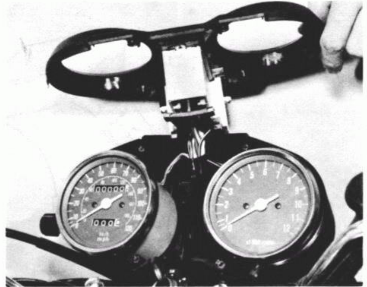
27.1b ...to enable the top section of the instrument console to be fitted
