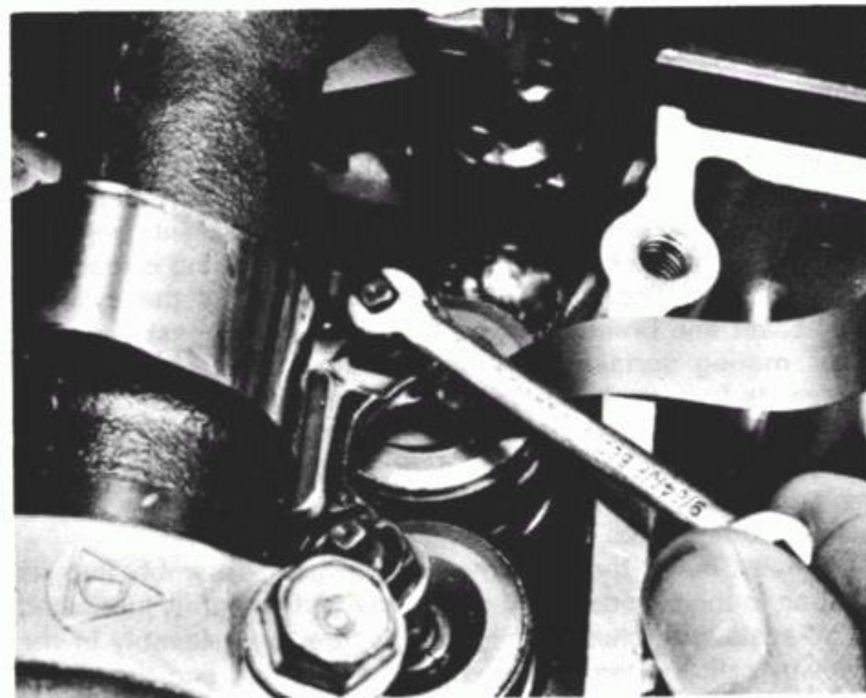
44.3a Turn the rocker arm adjuster whilst checking the valve clearance with a feeler gauge
