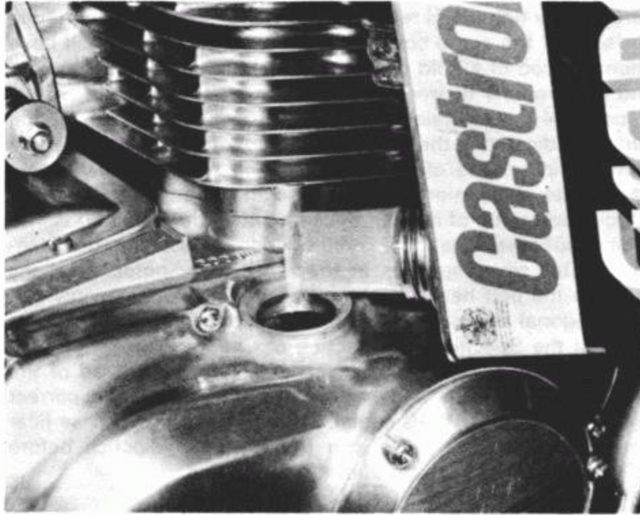
16.12a Pour the correct amount of recommended oil through the crankcase filler point...
