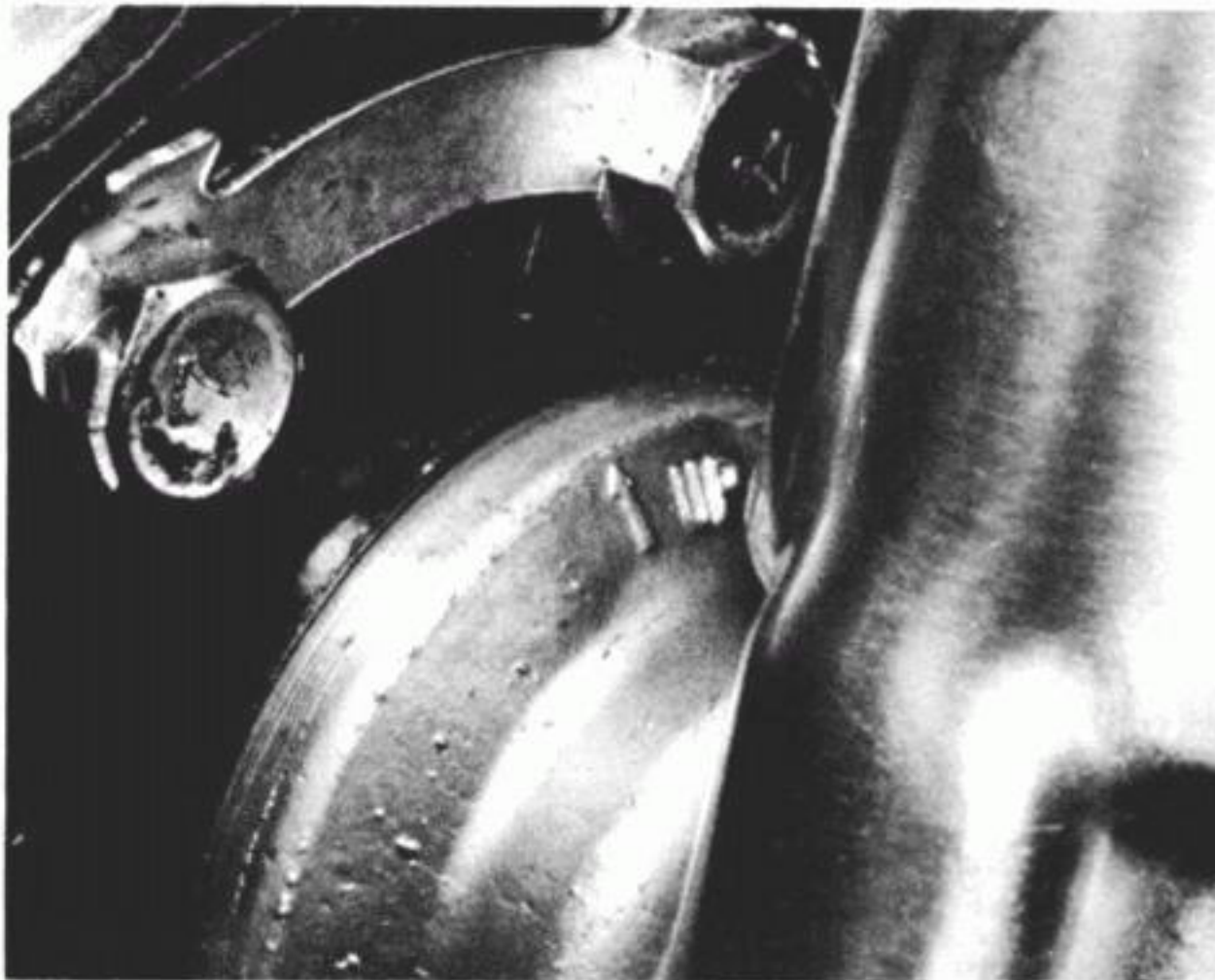
3.5e The embossed arrow-mark on the gearbox casing must point upwards
