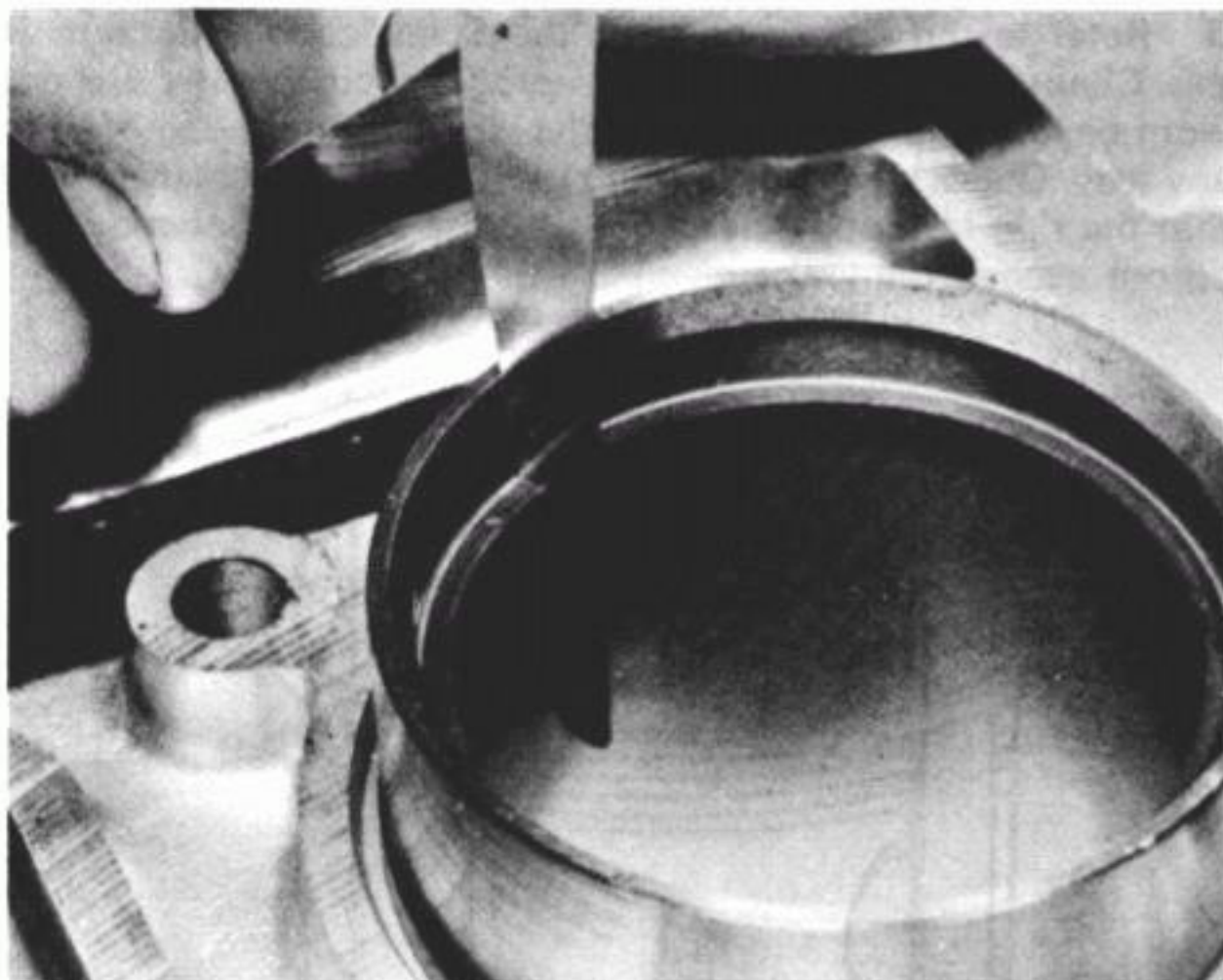
21.7 Measure piston ring wear as shown
