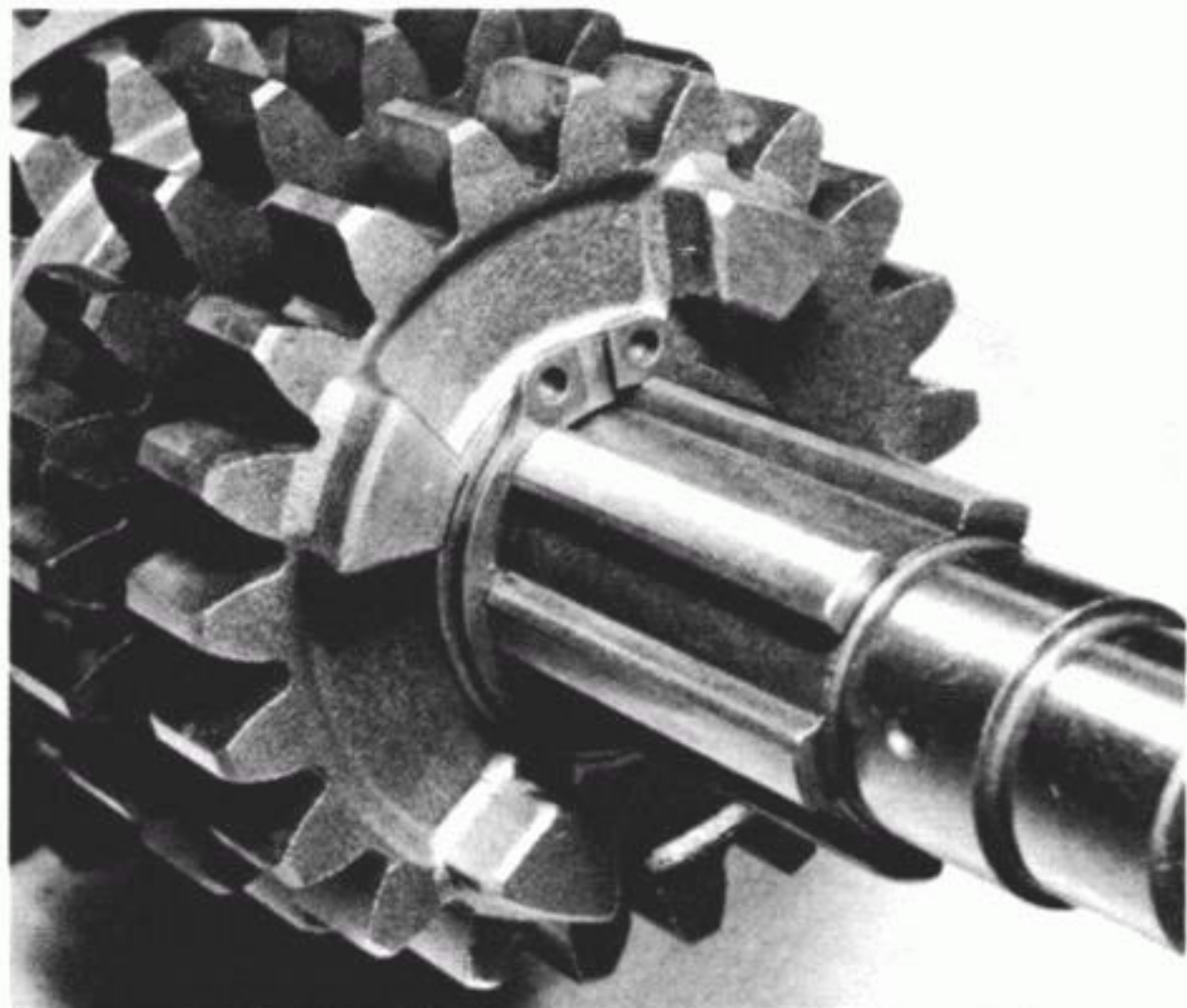
28.8o ...the 4th gear pinion, with its washer and retaining circlip...
