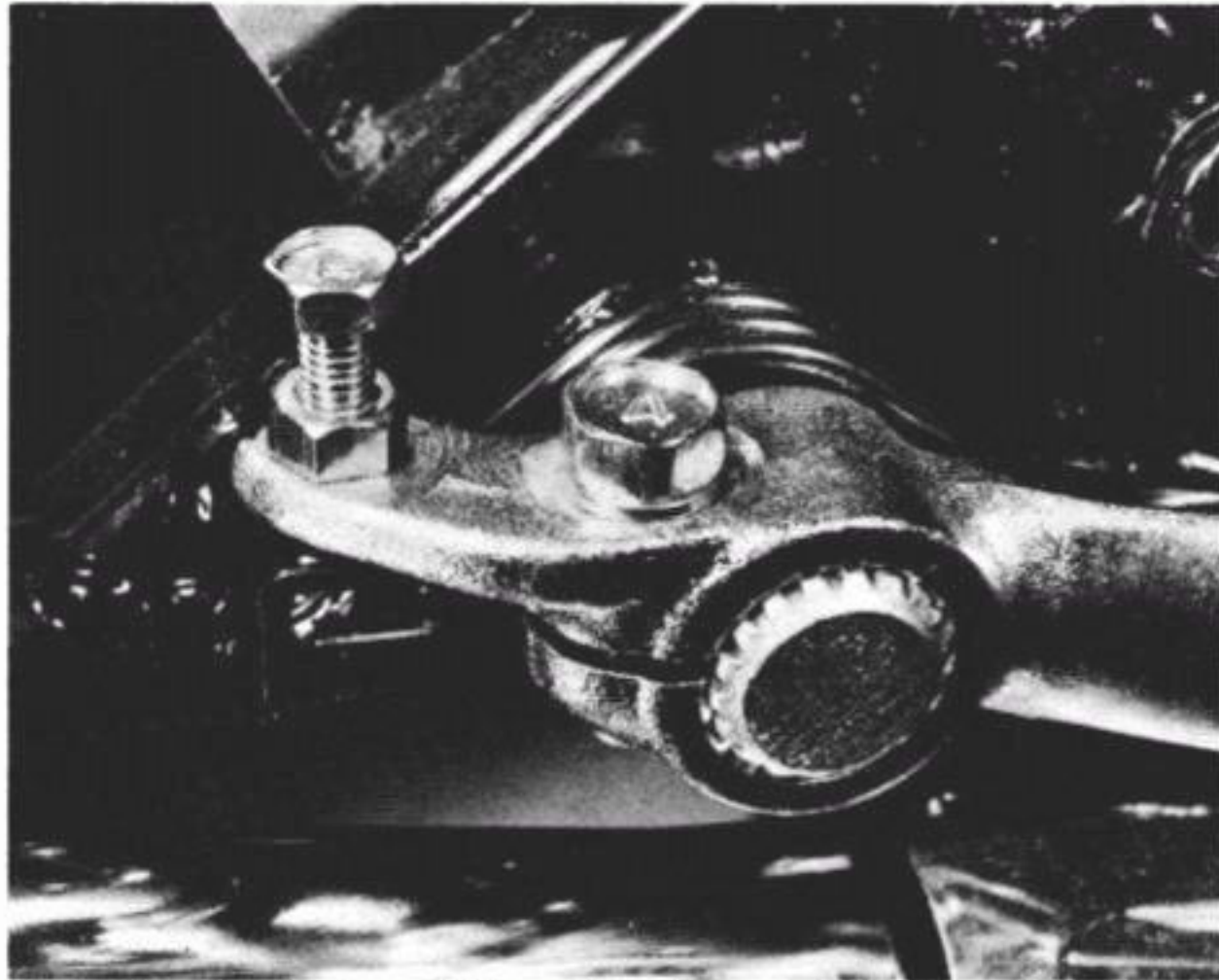
14.2 Alter the brake pedal position by rotating the adjuster bolt
