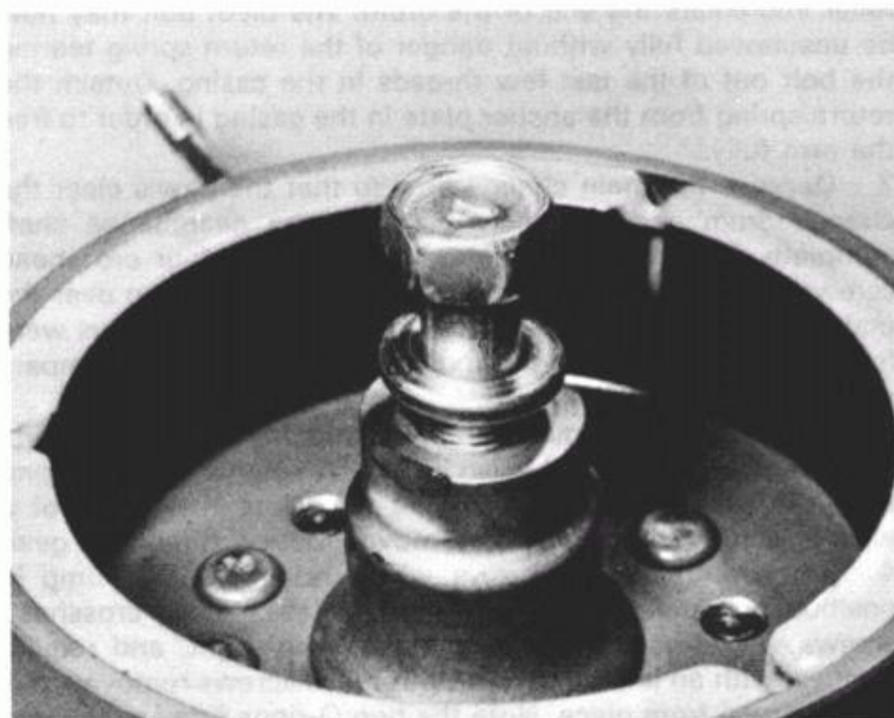
8.6a Remove the alternator rotor retaining bolt and washer...
