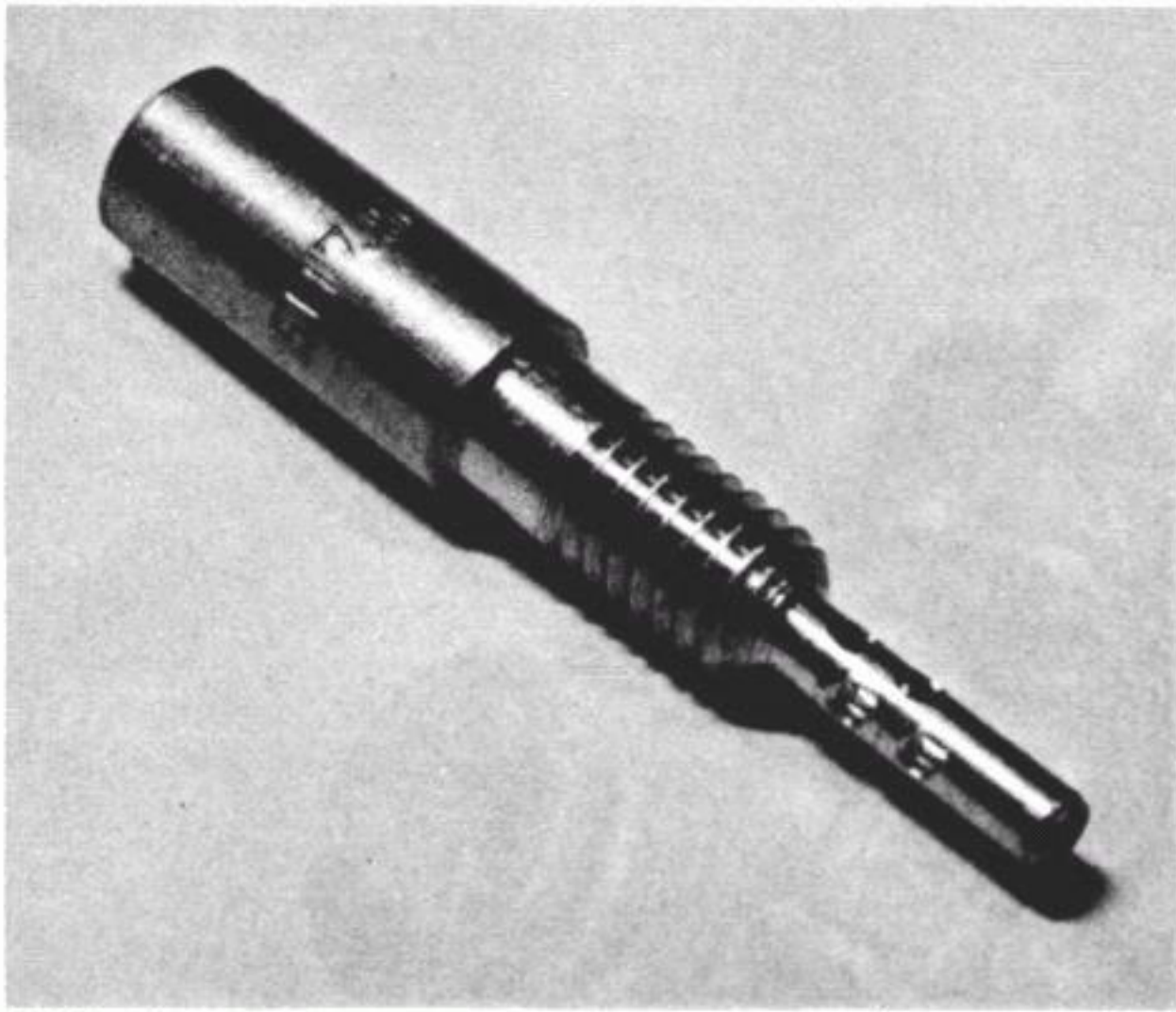
6.15a Thoroughly clean all components in fuel (pilot jet shown)...
