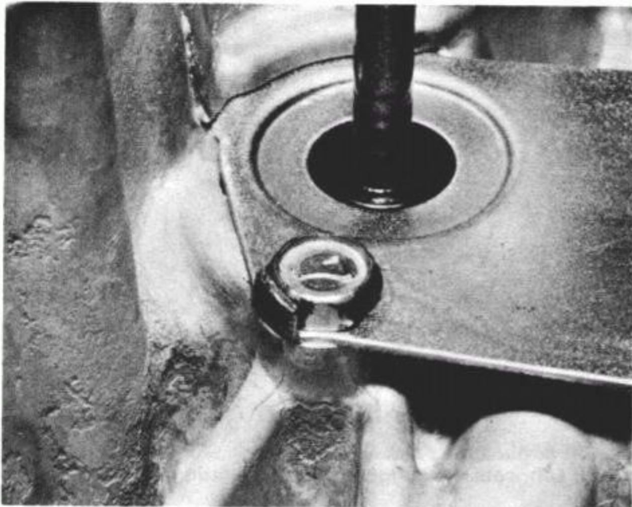
40.7 Lock the oil seal retaining plate (where fitted) bolts by bending up the plate tabs as shown
