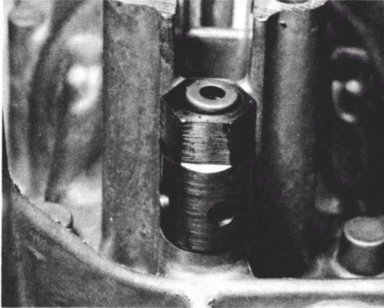
27.1b ...hooking out the spring retaining cap...
