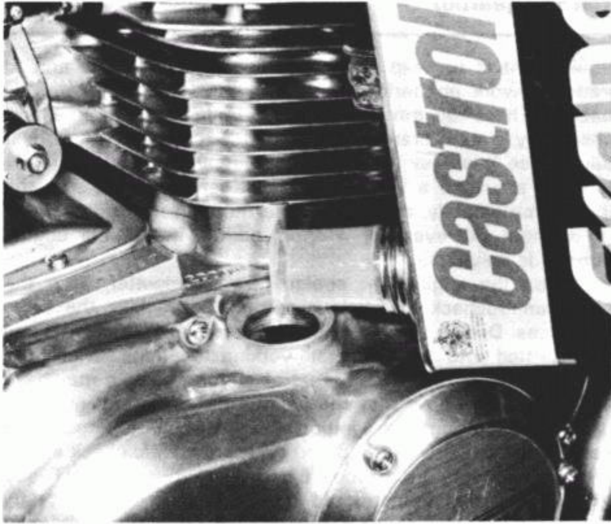
47.1a Replenish the crankcase with the correct oil...
