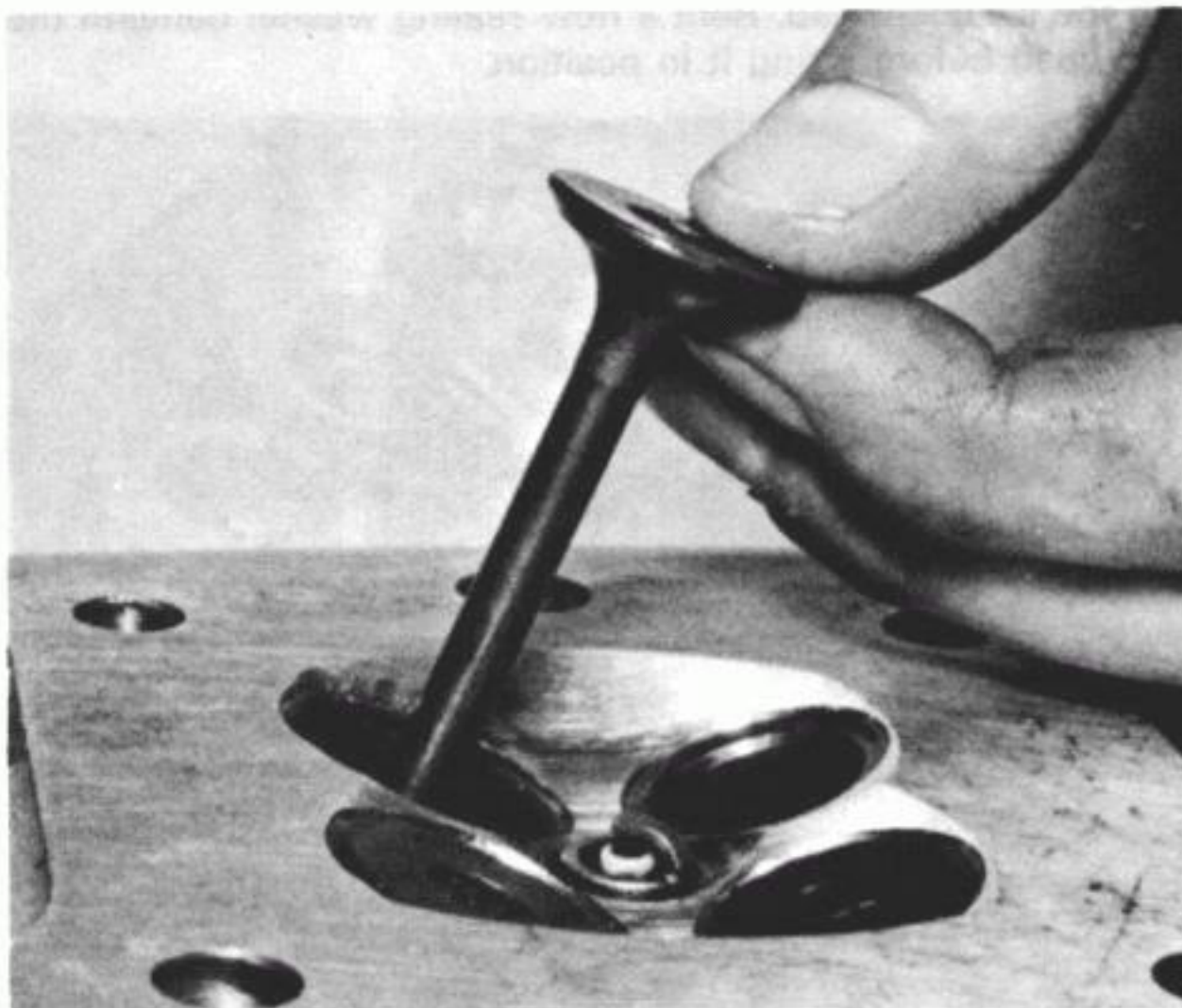
22.19b ...before lubricating and inserting the valve
