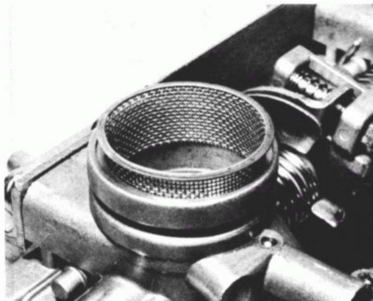
6.24b Where fitted, the atomiser ring should be relocated in the carburettor mouth
