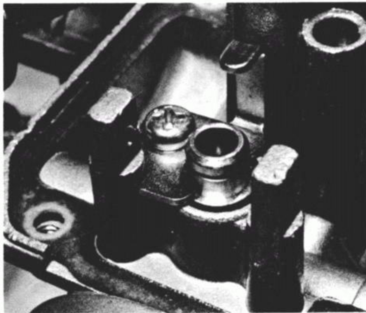
6.22g ...and fitting the needle seat retaining plate and securing screw
