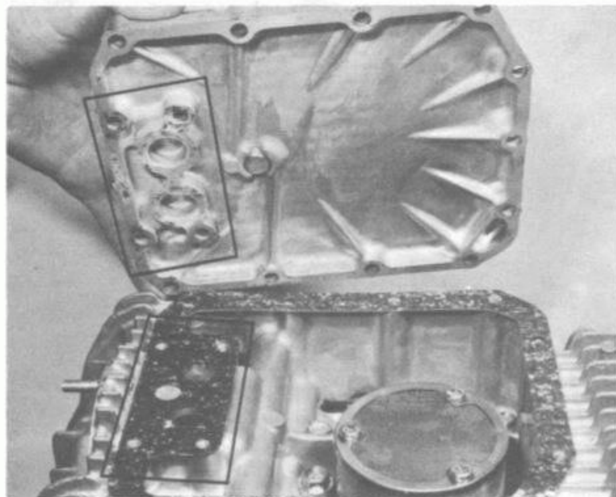
Smear an even coating of Suzuki Bond No 4 over the indicated crankcase and sump cover mating surfaces before fitting a new gasket
