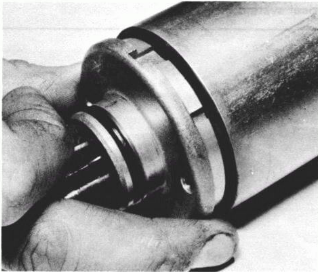
10.10b Refit the end cap with its serviceable O-ring...
