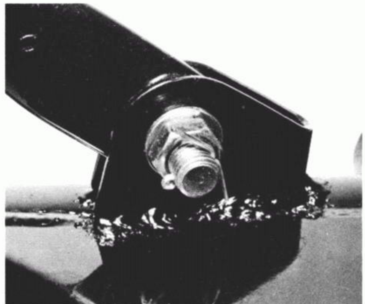
9.11e Check the torque arm to swinging arm connection for security...
