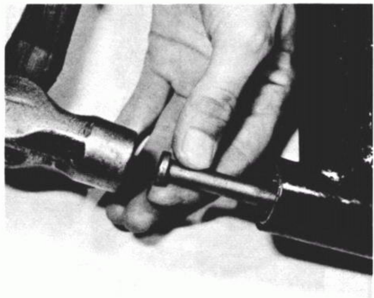
9.8b Use a length of steel rod to drift worn or damaged bearings from position...
