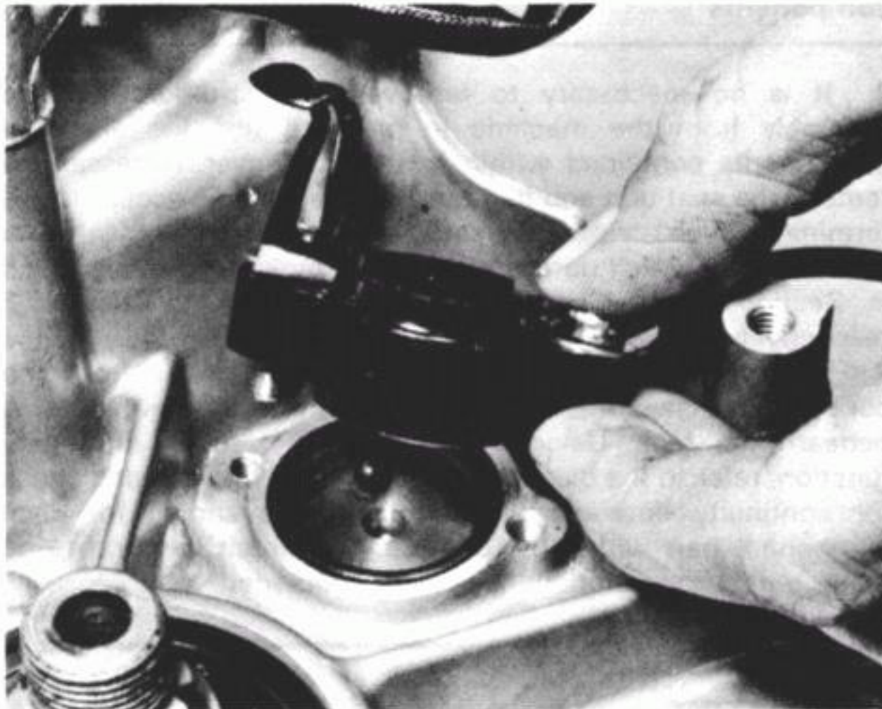
15.3 The O-ring fitted beneath the neutral indicator switch should be renewed whenever the switch is removed
