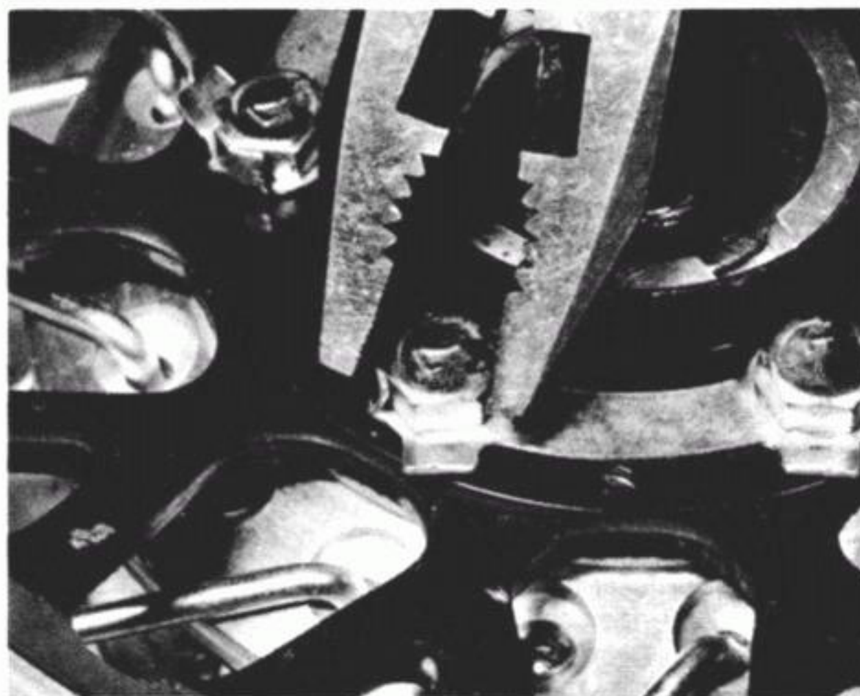
10.4 The brake disc securing bolts must be locked in position with the tab washer ends as shown
